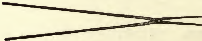
FIG. 12.—Crucible tongs for use in gasoline melting-furnace.
