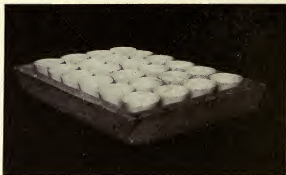
FIG. 21. — Clay dish holding 24 annealing cups.
