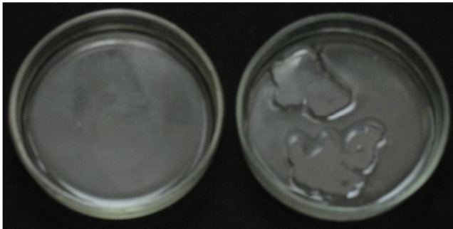
Figure 3. Left: 5 ml of water with an electric potential of -200 mV cover all the bottom of a Petri dish. Right: 5 ml of water with an electric potential of +200 mV do not cover the bottom of a Petri dish; the surface of such water decreases rapidly after mixing [10].
