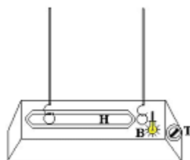
H Heater B Bulb T Theromostat
