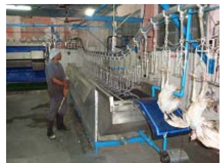
Fig. 4.7: Shackling of birds for slaughter Fig 4.8: Mechanized slaughtering of birds
