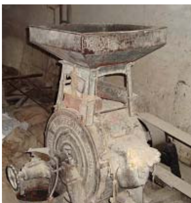
Fig. 2.3: Hammer mill
