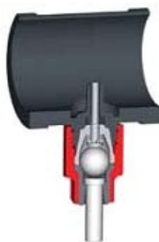
Fig. 3.17: Nipple assembly
