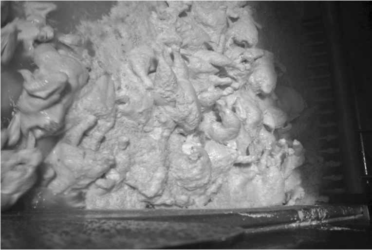
Figure 21.3 Exit of a chiller with water containing high levels of fat due to overscalding.
