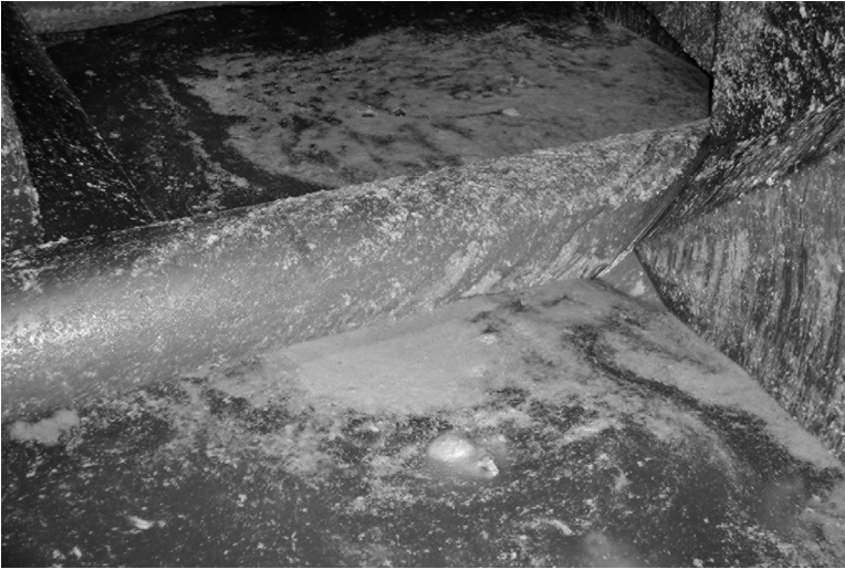
Figure 21.1 Chiller water containing high levels of organic material in the form of fat, blood, and protein.
