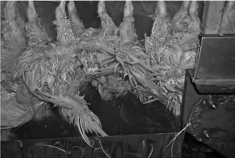
Figure 13.12 Water droplets coming off of the carcasses show that the scalding water at the scalding exit is clean.
