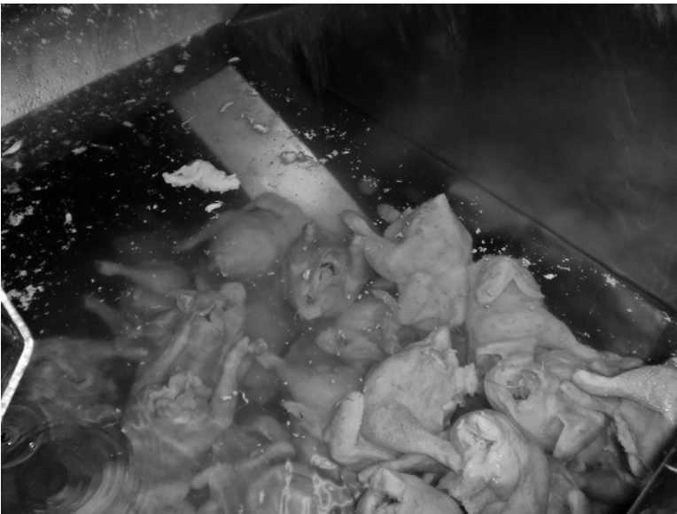
Figure 21.7 This is a chiller in Chile that is operating perfectly with extremely low organic loading at the chiller exit.
