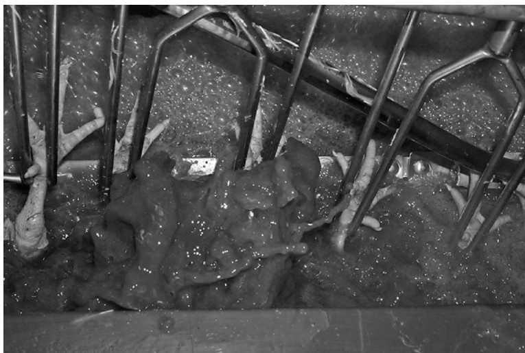
Figure 13.11 A scalding tank that is not operating in a countercurrent fashion showing filthy scald water.
