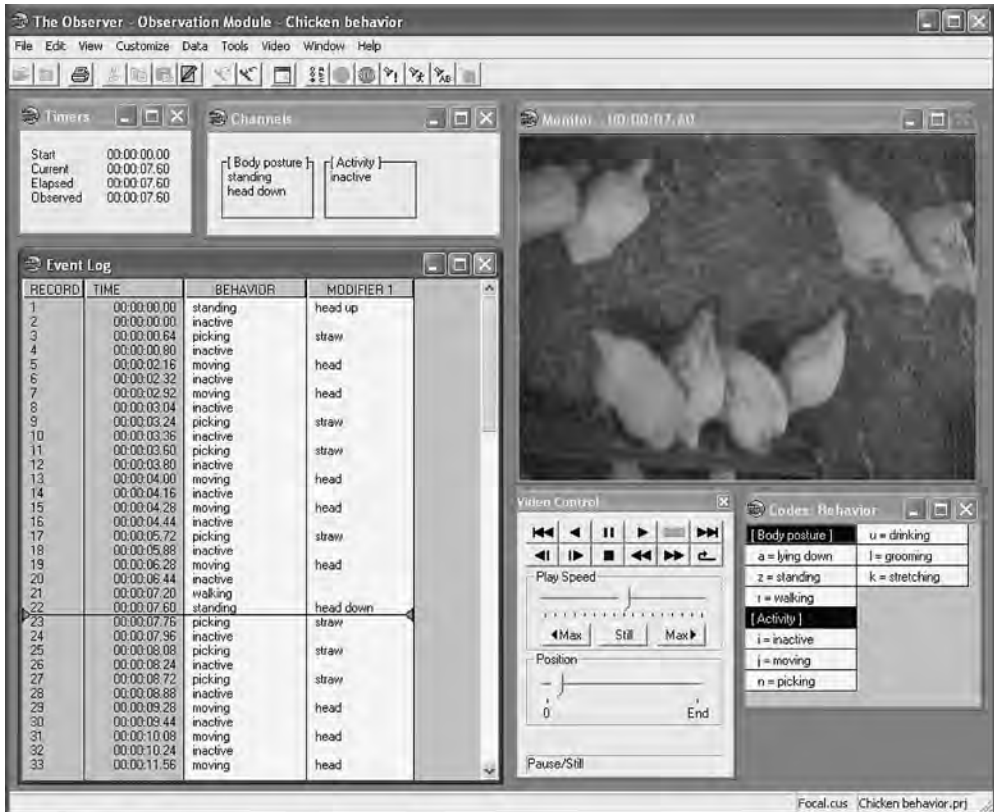
Fig. 23.2. Screen of THE OBSERVER during an observation session. The Event Log window contains the chronological list of observed events. The horizontal cursor indicates the time that corresponds with the current position in the video file, displayed in the Monitor window. (Video material by courtesy of M. Picard.)
