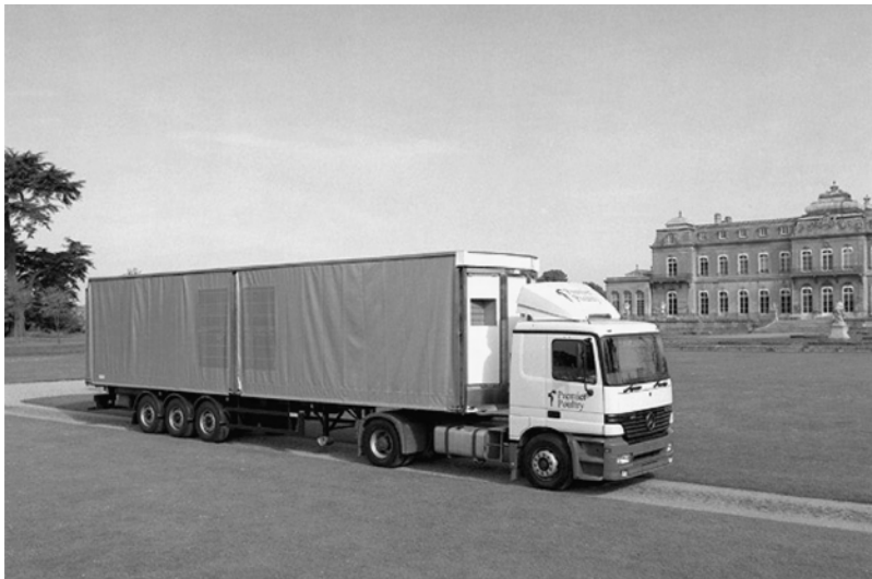
Fig. 12.2. Concept 2000, a mechanically ventilated broiler transport vehicle with automated control, now in commercial service.
