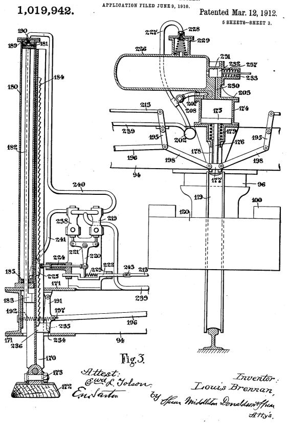
MEANS FOR IMPARTING TO AND MAINTAINING THE STABILITY OF BODIES SUCH AS SINGLE TRACK VEHICLES OR VESSELS.
