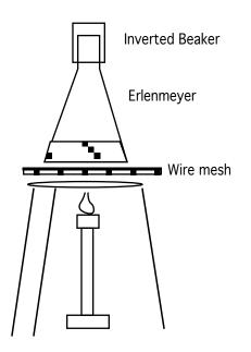
Figure 1. Heating liquid in Erlenmeyer Flask. Do not cook your thermometer.
