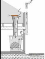
Schematic diagram of a Multi Chamber, Batch Cycle System
