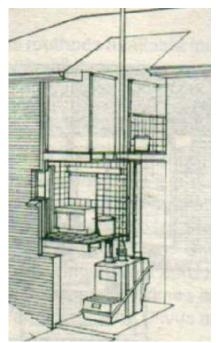
Schematic diagram & illustration of a Single Chamber, Continuous Cycle System
