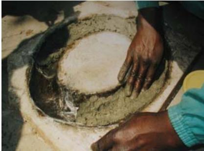
Figure 5-3: Adding concrete to the toilet seat mould
