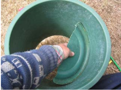
Figure 6-11: The cut base fitted half-way up the bucket at an angle
