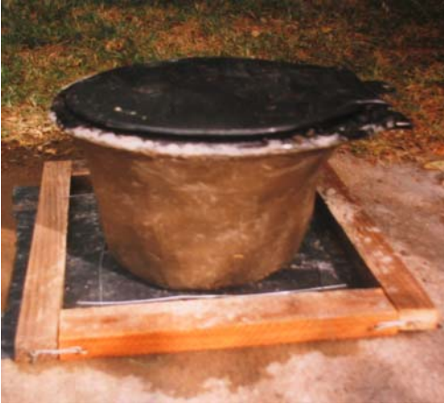
Figure 5-11: Completed pedestal placed in wooden mould
