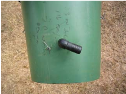
Figure 6-13: Fitting of the pipe bend to the bucket
