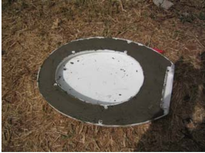
Figure 6-17: Concrete added to the toilet seat
