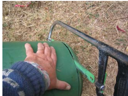
Figure 6-8: Cutting the base off the bucket
