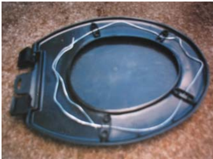
Figure 5-7: Ring of wire added to plastic toilet seat
