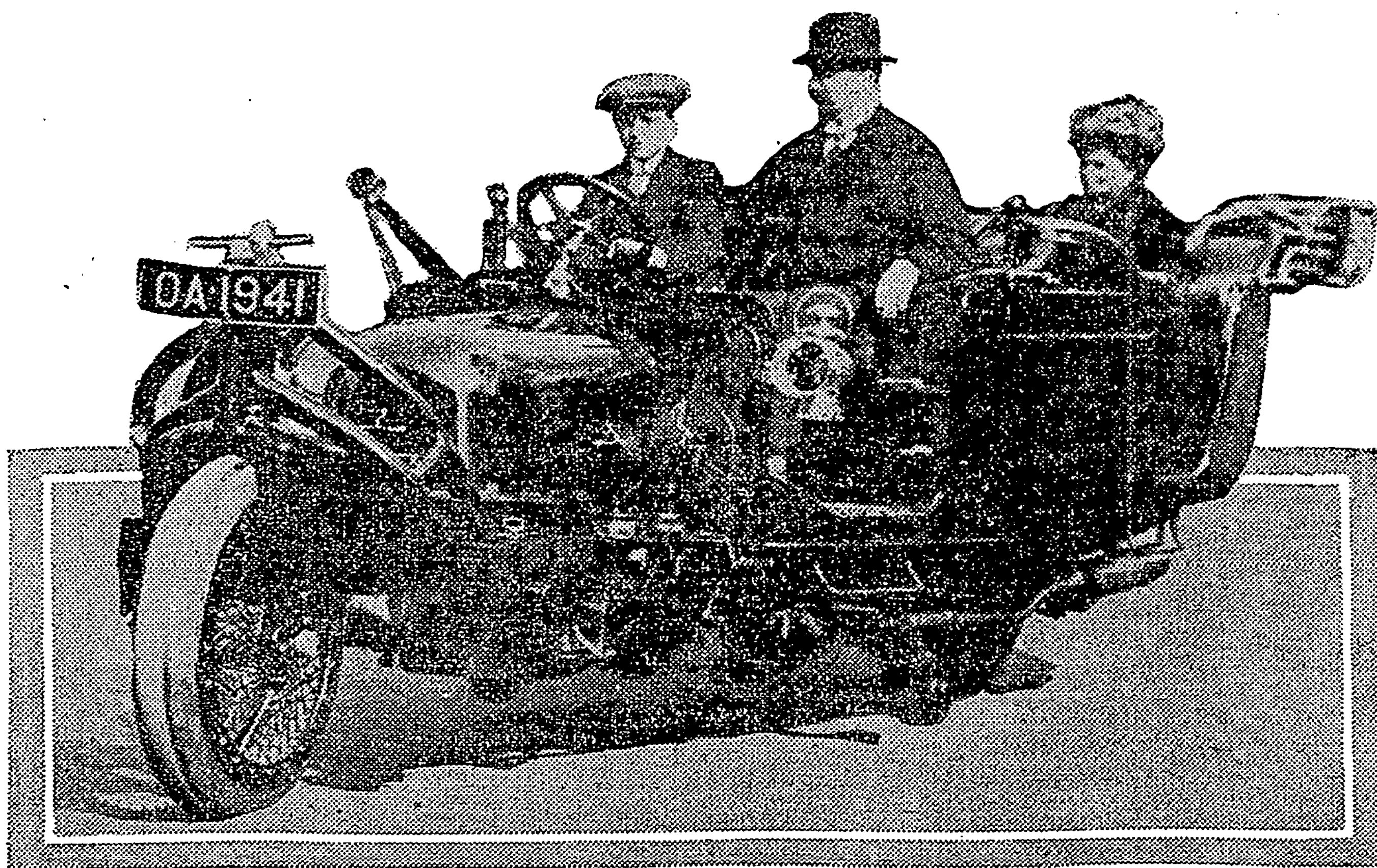
The gyro car which recently caused a sensation in London is here shown. It is the invention of Dr. Schilowsky, and is an odd contrivance in all its lines. Note the two little side wheels for emergency. (Photo copyright The Motor, England.)
