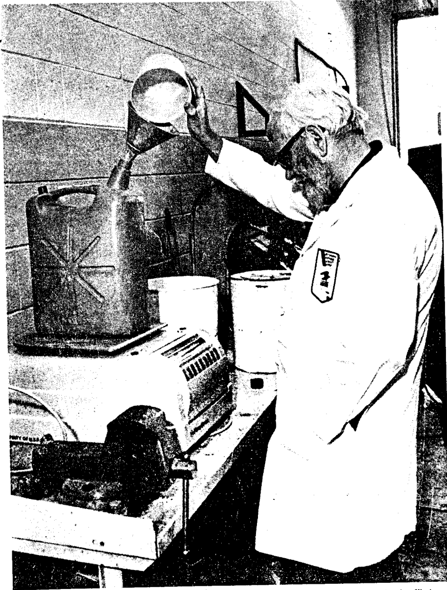
Emulsifiers—chemicals that allow water and gasoline to mix thoroughly—are essential to making watered fuel efficient. Here Ewbank weighs them out.
