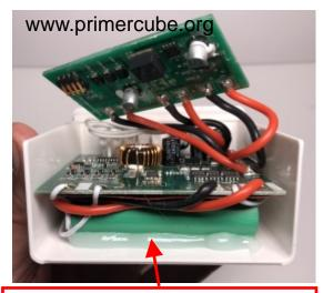
A bead of GE 5100 is used to secure batteries.
