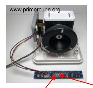
Follow these instructions to calibrate the Barmeter display. You will need to go through the high and low speed adjustments a couple of times as the POT settings affect each other.
