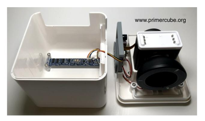
Place PC 7100 next to the lower PrimerCube assembly and connect the barmeter display to the motherboard with the 4 wire connector.
