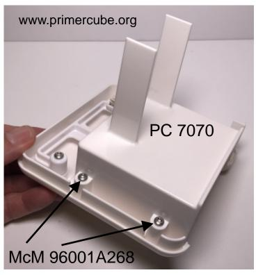
Attach PC 7070 to PC 7000 using 4 screws as shown. Use care not to overtighten screws as this can lead to part failure.
