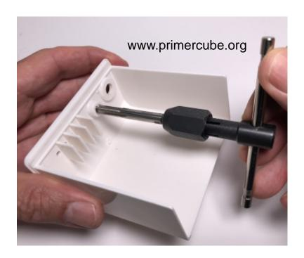
The image above shows part # PC 7010 and the hole for the pushbutton being tapped with a 1/4"-32 bottoming tap. Only tap the hole deep enough for the pushbutton or the outside of the hole will appear cosmetically irregular.
