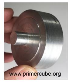
Above are three views of a aluminum fixture used to press the Maxon motor into PC 200. The small magnet in the fixture holds the Maxon motor while pressing it into place.
