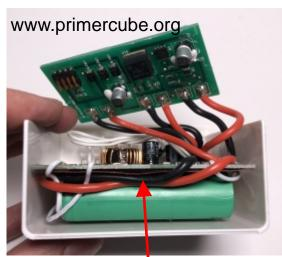
Secure wires in place with Loctite 401 adhesive.
