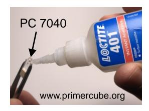
Hold PC 7040 with tweezers and apply Loctite 401 sparingly as shown above. Then carefully insert PC 7040
