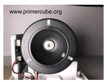
Next the .10 gram of clay is moved to location 2 and the vibration level is measured while the rotor is running at full speed. (3350 RPM)
