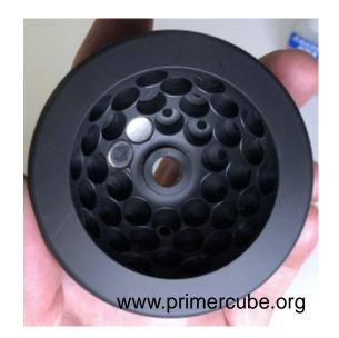
Repeat the process for the second magnet and for each magnet thereafter in the inner ring of magnets. Repeat this process for the second ring, then the third ring and then the fourth ring of magnets until the all 40 magnets are glued in place. This entire process takes about 15 minutes to do by hand but could be done by an automated machine in five minutes or less.
