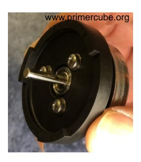
Place the screw into the hole and tighten firmly but do not over tighten. Repeat the process for the other two screws. This photo shows the motor with Part # PC 8700 attached with the three screws.
