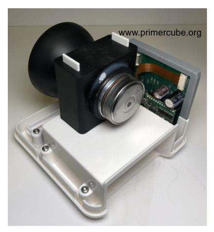
Take the rotor assembly from the prior steps in this manual and place it in position as shown in the photo to the left. Attach the ribbon connector to the PrimerCube Motherboard as shown.
