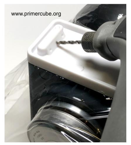
Using a .077 inch diameter drill bit make six holes in the locations indicated by the marks on PC 8600. The holes should be about ½ inch deep. Keep the drill bit at 90 degrees to the surface with the location marks as shown in the photo.
