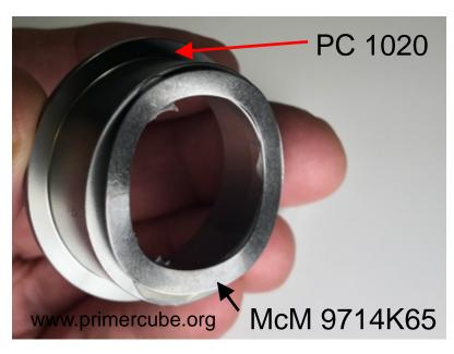
Attach McM 9714K65 (Wave Spring) in place with GE5100 Silicone Sealant onto the second PC 1020.
