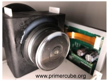
Then the temporary clay weight is removed from the motor and the same amount by weight of GE5100 silicone is used as the permanent balancing weight. The silicone must set for at least 30 minutes before running the rotor again. A final vibration measurement is taken and adjustments to the holes or the silicone are made if needed for a smooth running rotor. Self adhesive balancing weights are another option if used properly.
