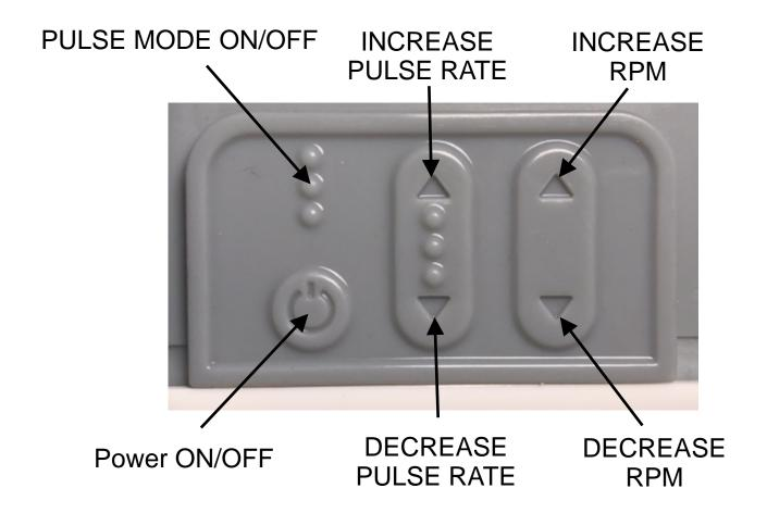
The keypad on the side of the PrimerCube is shown above.
