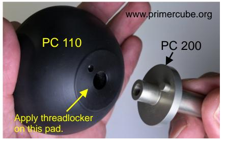
Insert part # PC 200 into the backside of part # PC 110 making sure to align the small pin with the matching hole. It is desirable to put some threadlocker between these two parts to insure that there is no movement after assembly and curing.
