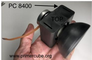
Above are two views of the completed rotor assembly ready for balancing after allowing 24 hours for curing. Once again notice the proper orientation of the motor leads and PC 8400.
