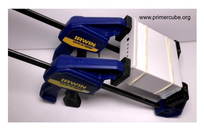
Apply clamps and squeeze out excess GE 5100 silicone. After allowing the silicone to cure for three hours the excess silicone can easily be removed. This completes the battery pack.
