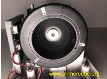
A hole or holes if needed are drilled 180 degrees from the temporary clay balancing weight. Then the temporary clay is removed and the rotor is run at 3350 RPM. The vibration level is measured to see if it is the same as with the temporary clay weight. If needed then the hole can be drilled deeper or more holes can be drilled until the vibration level is equal to that achieved with the temporary clay balancing weight.
