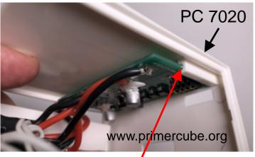
Slide the small PCB into the slots as shown and secure with a drop of Loctite 401 on each side.
