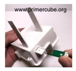
Place the DC Input Mini PCB into location shown and attach with screw McM 96710A215
