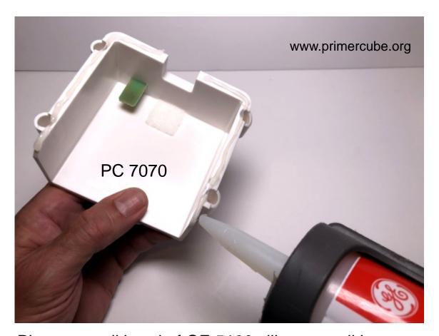
Place a small bead of GE 5100 silicone caulking as shown in photo above.
