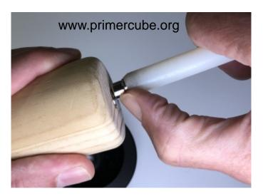
Use magnet insertion tool to remove one magnet from the stack.
