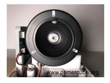
Then a .10 gram of clay is placed at position 1 and the vibration level is measured while the rotor is running at full speed. (3350 RPM)
