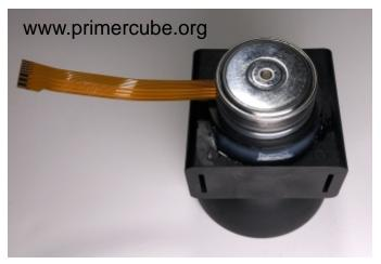
After pressing the Maxon motor into place put a small amount of GE 5100 or equivalent as shown above. Skipping this step can lead to undesiredable vibration when the unit is running. Before running this assembly it should then set for 24 hours to allow the curing of the threadlocker, the Loctite 648, and the silicone.
