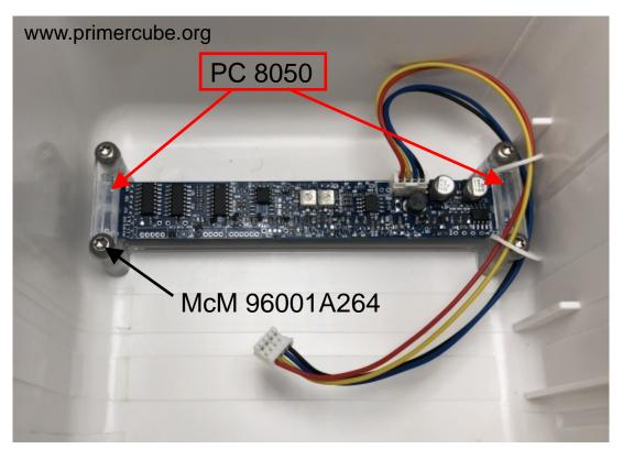
Place the two PC 8050 in position shown and secure with four McM 96001A264 screws. Do not over tighten these screws as it will result in stress cracks in PC 8050. Thread the 4-wire connector through the rubber bands.
