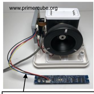
Next connect the barmeter display to the PrimerCube Motherboard using the 4-wire connector as shown above.
