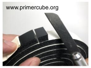
Cut a piece of 1/4" x 3/4"self adhesive foam rubber weatherstripping 1/2" long.
