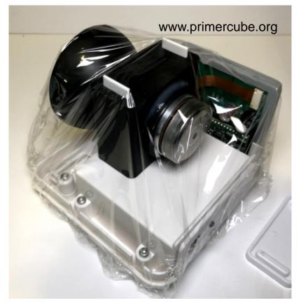
Wrap the entire assembly in plastic wrap to keep shavings and debris from getting into critical parts during the steps to follow.
