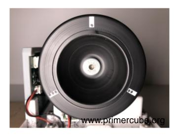
Above we see the rotor marked in three spots 120 degrees apart. The vibration level is measured while the rotor is running at 3350 RPM
