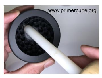
Insert the magnet into the hole until it bottoms out and then hold for a few seconds to allow the adhesive to cure.
