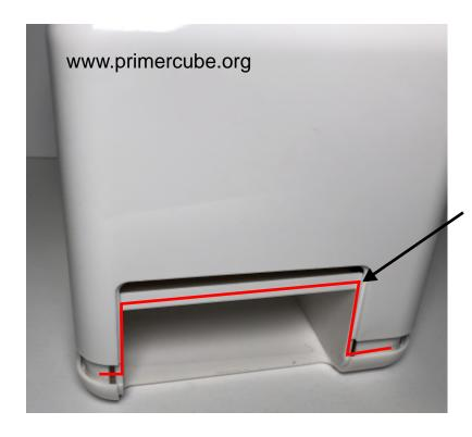
Also place a bead of GE 5100 silicone sealant in the area indicated in red.
