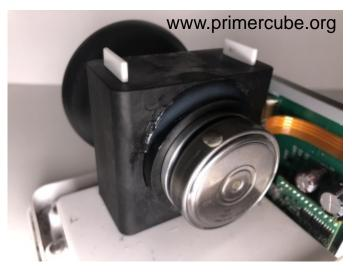
After a bit of fine tuning we have the proper weight and location of the two temporary clay balancing weights required for a smooth running rotor. The photo to the right shows the temporary balance weight on the motor, but some rotors do not need this balancing weight as they are smooth enough with just the balancing weight on one side of the bearings.
