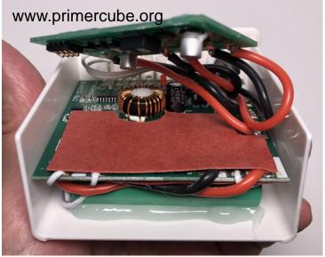
Place self adhesive insulating paper over the area of the lower PCB shown above.
