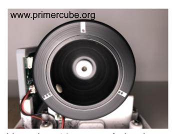
Next the .10 gram of clay is moved to location 3 and the vibration level is measured while the rotor is running at full speed. (3350) RPM) We are not providing the complete instructions on proper use of the iRotorBalance app to balance the rotor assembly as this guide is intended for manufacturers who will most likely not use this app.
