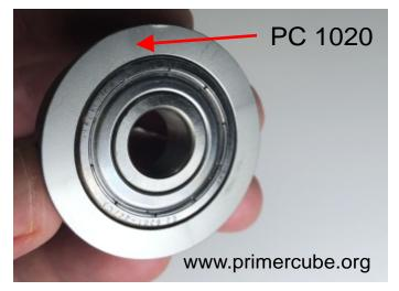
Place bearing part # SKF E2.6201-2Z/C3 into PC 1020 and press until fully seated. Each bearing should be checked to make sure that it is running freely and smoothly without any rough spots before it is pressed onto PC 200 Shaft. A drawing for the specifications of PC 1020 is available in the Technology Transfer area at www.primercube.org.
