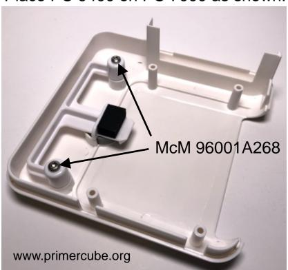
IMPORTANT! Attach using screws being careful to not over tighten as this will keep the assembly from seating correctly.
