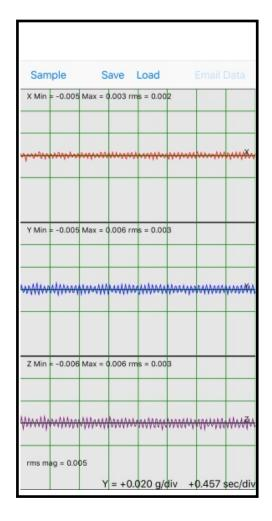
To the top left is a screenshot of the desired vibration readings using the Vibration app on the iPhone. These readings were obtained using the simple setup shown in the image below.
