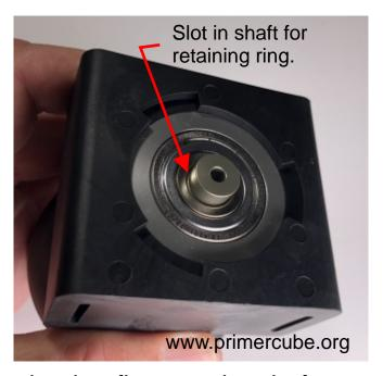
Using a hydraulic press and a tube that fits over the shaft, press the bearing into the proper position.
