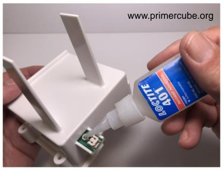
and nut McM 91841A005. Use Loctite 401 as threadlocker. IMPORTANT! Avoid threadlockers that can cause stress cracking on plastic parts and result in part failures. We have found Loctite 401, although not technically a threadlocker, to work very well and also not cause stress cracking.
