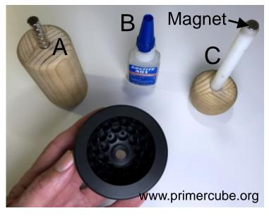
Shown in the photo to the left are the items used to glue the magnets into the bowls by hand.
