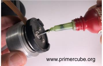
Place a small drop of Loctite 648 into the hole on the end of the shaft of PC 200 and a small amount around the shaft on the Maxon motor. Carefully avoid using excess Loctite 648 so that it does not drip off and cause issues with the motor or bearings.
