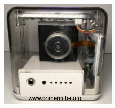
improving functionality at the same time. It is important to note that the barmeter display on the PrimerCube indicates the actual running speed of the rotor through hall sensors in the Maxon motor. A smart phone/tablet interface needs to receive this information in real time to enable the user to monitor the actual running speed of the rotor. This is important as this insures the user is receiving the "dosage" from the PrimerCube that they believe they are.
