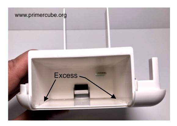
Excess silicone caulking should be removed .
