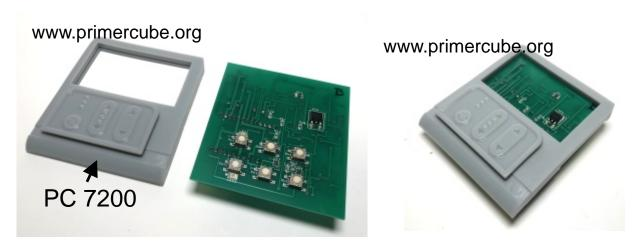
Insert PrimerCube Motherboard into PC 7200 and then place into PC 7000 as shown below.
