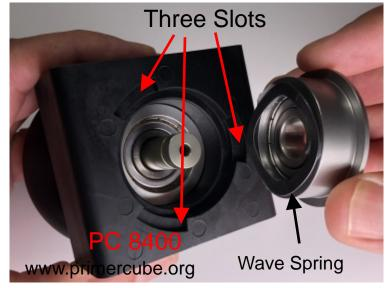
Insert the assembly from the previous steps into PC 8400 as shown above paying careful attention to the orientation of PC 8400. Then place the bearing assembly with the wave spring attached onto the shaft as shown. Only one wave spring is used in this assembly.
