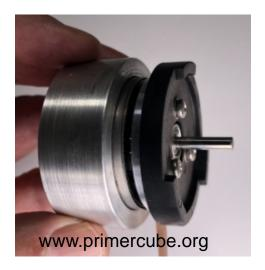
The two images above show how the Maxon motor fits into the aluminum fixture used for pressing the motor into PC 200.
