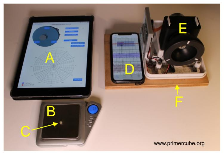
The image above shows the items required to balance the rotor assembly in about 20 minutes per unit. A custom balancing machine should be used for large production as that would greatly reduce the time required per unit. Shown in the image above are:
