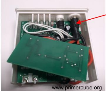
Place the input socket into the proper hole and secure with the washer and nut.
