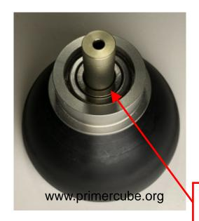
Bearing should be a press fit for the smoothest running assembly. The drawing for part # PC 200 on <a href="www.primercube.org">www.primercube.org</a> specifies a shaft diameter for the correct press fit.
