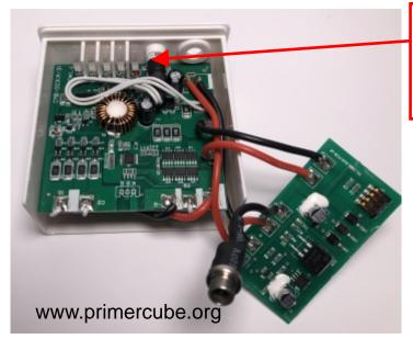
Thread the pushbutton into the tapped hole and then slide the PCB and attached batteries into place as shown.
