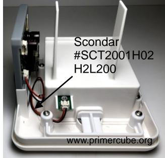
Connect PrimerCube motherboard to the DC Input PCB using Scondar part # SCT2001H02 H2L200.
