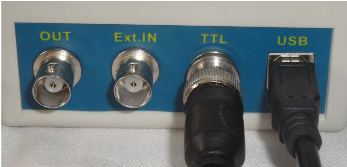
Fig. 2: Connector block of the DDS generator (on the back)
