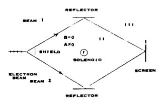
Fig. 1 Set-Up for Aharonov-Bohm Interference Experiment
