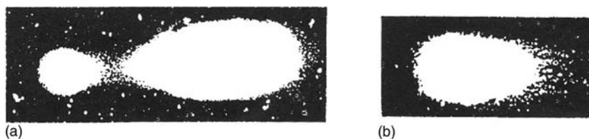
Figure 34.4 Typical DNA comets from (a) irradiated (at 7.5 kGy) and (b) nonirradiated tissues. (Haine, H., Cerda, H., and Jones, L., Food Sci. Technol. Today , 9(3), 139, 1995. Copyright IFST.)
