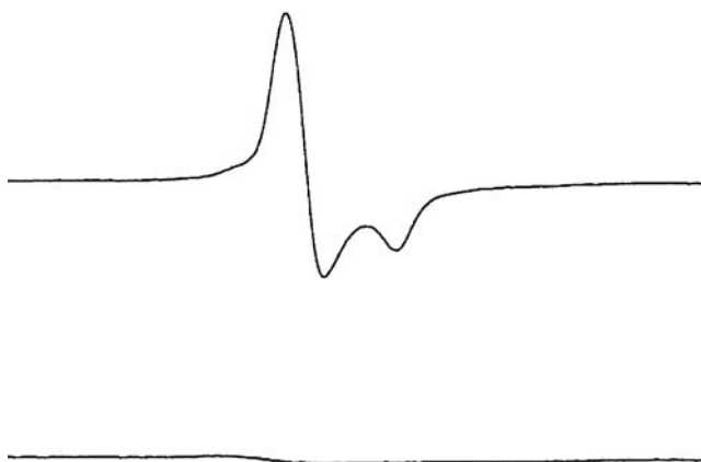
Figure 34.1 ESR spectra derived from irradiated (top spectrum) and nonirradiated (bottom spectrum) bone from frog legs.
