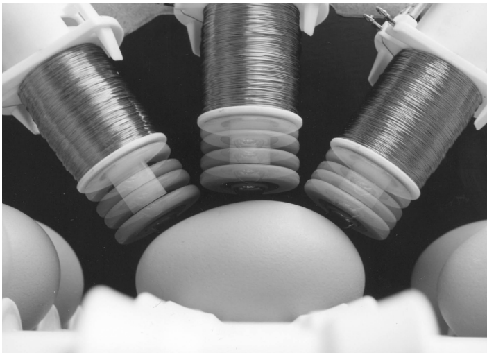
Fig. 10.16 Crack detection method of Moayeri (1996). Picture property of Moba BV.
