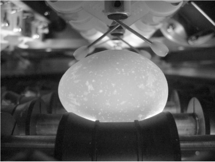
Fig. 10.15 Crack detection method used by Staalkat International BV and Nabel Co. Ltd. Picture property of Sanovo Staalkat Group.
