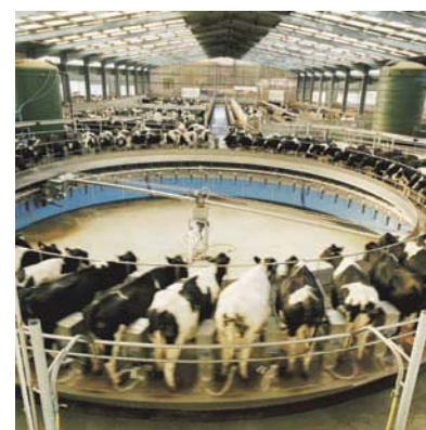
Figure 45-9 A rotary milking parlor rotates slowly as cows are milked. Courtesy of Getty Images.
