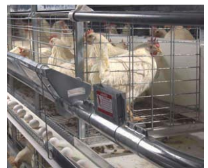
Figure 36-1 Eggs roll to the front of the layer cages and are moved on an automated system to the packing house. Courtesy of Chore-Time Poultry Production Systems, Milford, Indiana.
