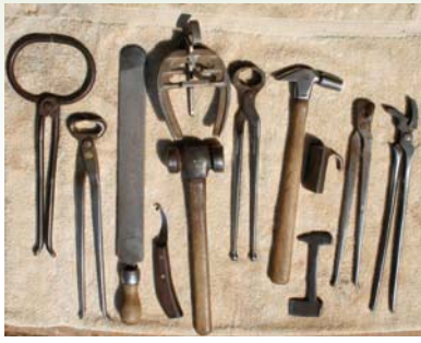
Figure 32-12 Tools used by a farrier (left to right): hoof testers, hoof nippers, rasp, hoof knife, hoof gauge, turning hammer, pulloffs, driving hammer, clinch pan, clinch cutter, crease nail puller, and clinchers. Photo by Dr. Frank Flanders. Courtesy of Wayne Nunn Farrier Service.
