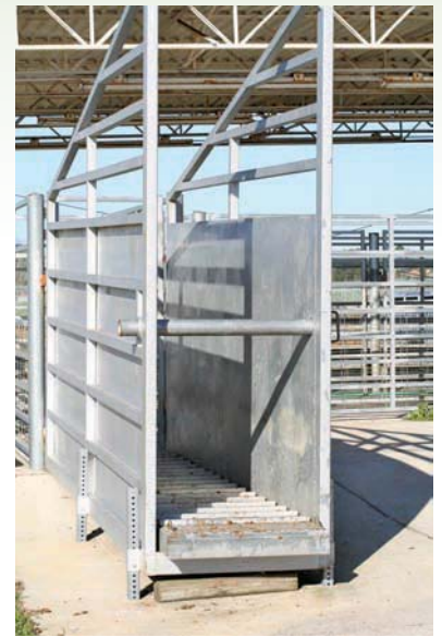
Figure 24-9 Modern adjustable chutes are used to load cattle, hogs, and other livestock. The platform can be lowered or raised depending on the height of the truck or trailer bed. Photo by Dr. Frank Flanders.
