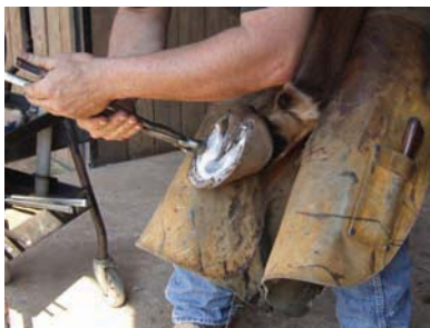
Figure 32-15 Nippers are used to trim the outer surface of the hoof to a proper angle and length to fit the conformation of the animal. Photo by Dr. Frank Flanders. Courtesy of Wayne Nunn Farrier Service.
