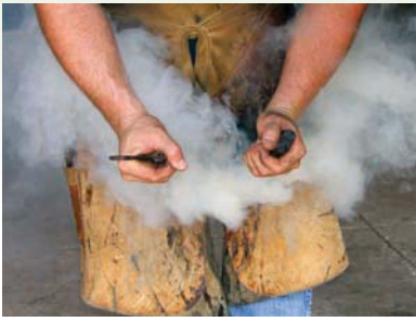
Figure 32-18 A farrier will often take a hot shoe from the forge and press it to the bottom of the horse's hoof. The slight burning not only shows the farrier where to make alterations to the shoe and smooths any uneven areas on the horse's foot, but it also helps kill bacteria that cause white line disease. This procedure does not cause any pain to the horse. Photo by Dr. Frank Flanders. Courtesy of Wayne Nunn Farrier Service.
