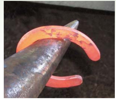
Figure 32-14 Horseshoes heated in a forge are moved quickly to an anvil for shaping. Photo by Dr. Frank Flanders. Courtesy of Wayne Nunn Farrier Service.
