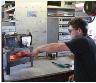
Figure 32-13 A farrier uses a forge to heat the shoe and make it easier to shape. Photo by Dr. Frank Flanders. Courtesy of Wayne Nunn Farrier Service.
