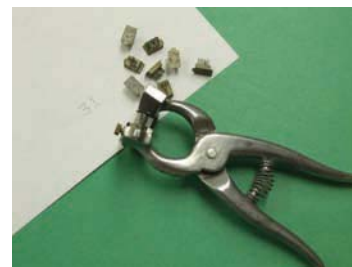
Figure 15-11A A simple type-tattooing instrument with interchangeable numbers and letters. Photo by Dr. Frank Flanders.
