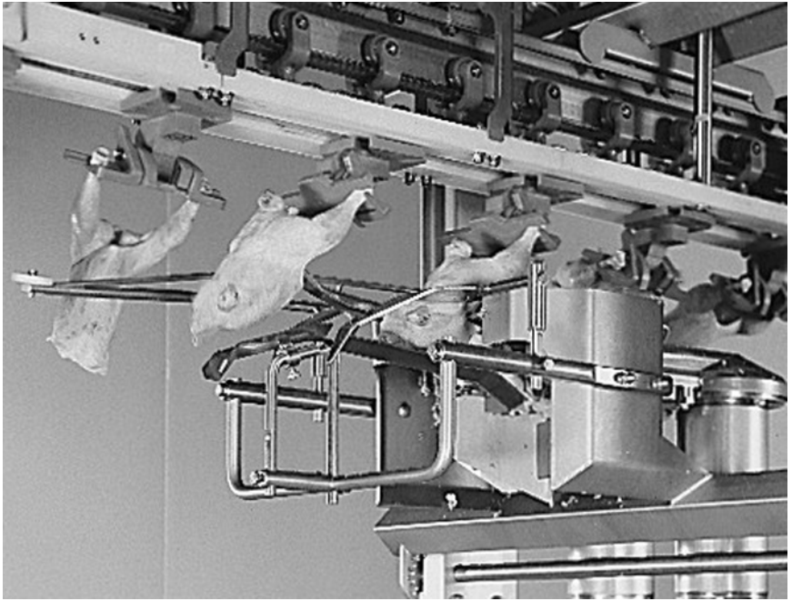
Fig. 5.7 Breastcap cutter with by-pass.
