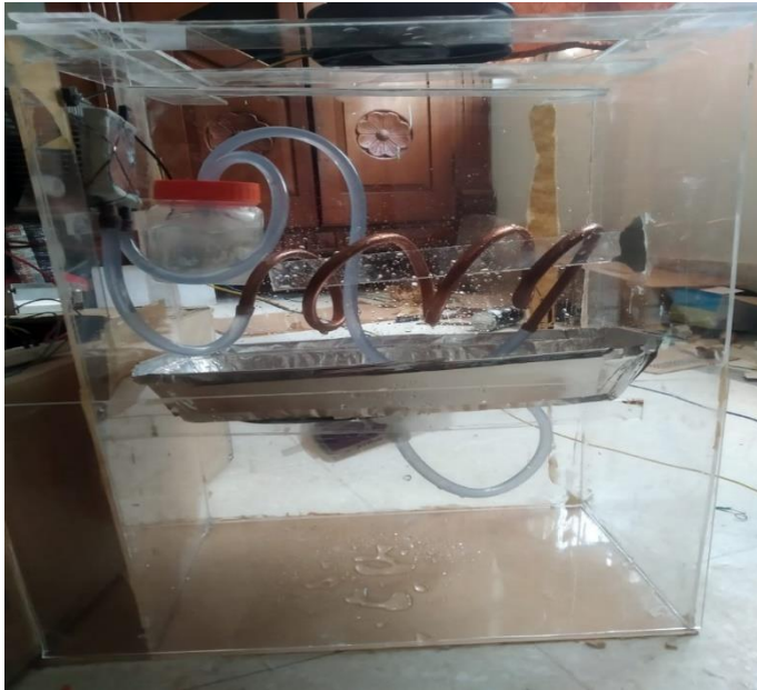
Fig.5: AWG system and water level control module
