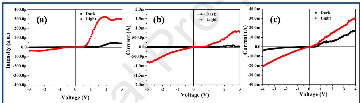
Fig.8. I-V characteristic of siloxene nanosheet for different thickness (a) 230nm (b) 600nm and (c) >1 $\mu$ m
