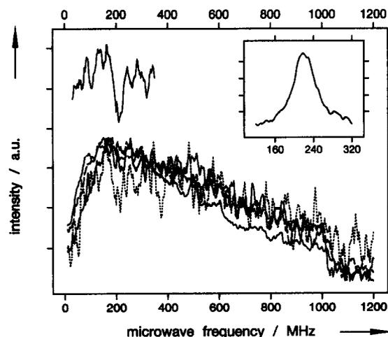
Fig. 4. Main figure: Zf-ODMR-signal of  $S_x(\text{an})$  at 4 power levels (2200 mW: —; 220 mW: - - ; 22 mW: · · — · ·; 2 mW: · · · ·), modulation frequency: 1030 Hz. Upper part left: sweep while hole burning cw power at 200 MHz, 100 mW. Upper part right: sweep with hole burning at 200 MHz, modulated with 1030 Hz, sweep power unmodulated. Optical excitation as given in fig. 2. Detection with a photodiode and  $\lambda_{\text{det}} > 550 \text{ nm}$ .
