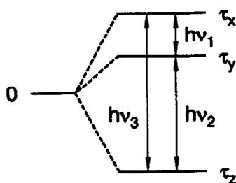
Fig. 1. Zero field splitting of the triplet state (schematically). The indicated transitions between the three possible spinfunctions  $\tau_i$  have the following energies:
