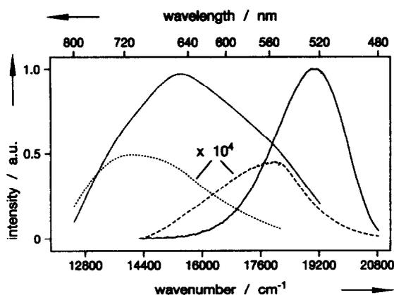
Fig. 2. Photoluminescence (PL) emission of Sx(ap) —, excitation at 457 nm, Sx(an) - · - ·, excitation at 360 nm. Both spectra are normalized to 1 at their peak intensity and corrected with the spectral sensitivity of the apparatus. The curves normalized to 0.5 represent the respective MIE spectra ( $\times 10^4$ , see text) of Sx(ap) - - - and Sx(an) · · ·. Excitation conditions as in case of the respective PL.
