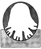
Stage 2: Foaming of slurry Stage 3: Coalescence of pores leads to cavity
