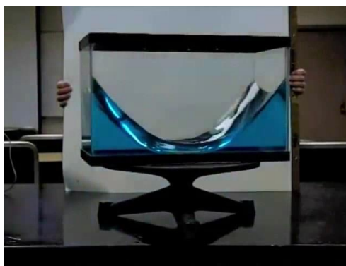
Fig. 1. Curvature of the water surface when the vessel rotates
