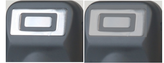
Electrode corrosion can occur If not cleaned regularly.
