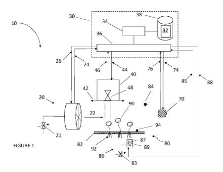
(57) Abstract: Embodiments of the disclosure relate to apparatus and methods for monitoring plant development in aeroponic farming. The output from one or more sensors in the apparatus be used to modify the flow of one or more fluids to the developing plants.
