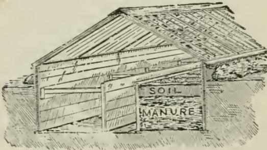
Fig. 16. Manure-heated forcing-house.
