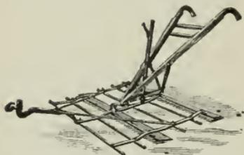
Fig. 33. Leveling device attached to a cultivator frame.
