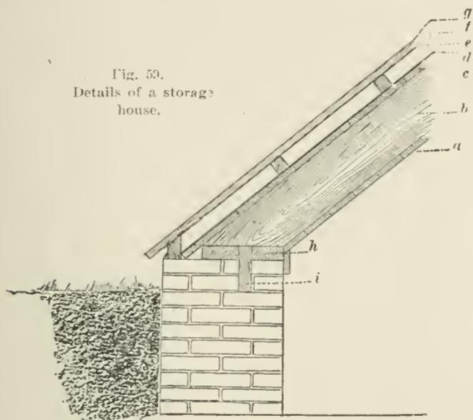
building paper at *d* and *f*. The cost of labor and materials is about \$500. An interior view of this house is shown in Fig. 57. It was stocked with celery at the time this picture was made, and in spite of having been harvested early, the plants were faring well.
