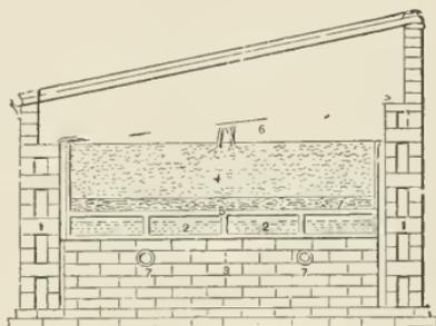
Fig. 17. Pipe-heated hotbed.
