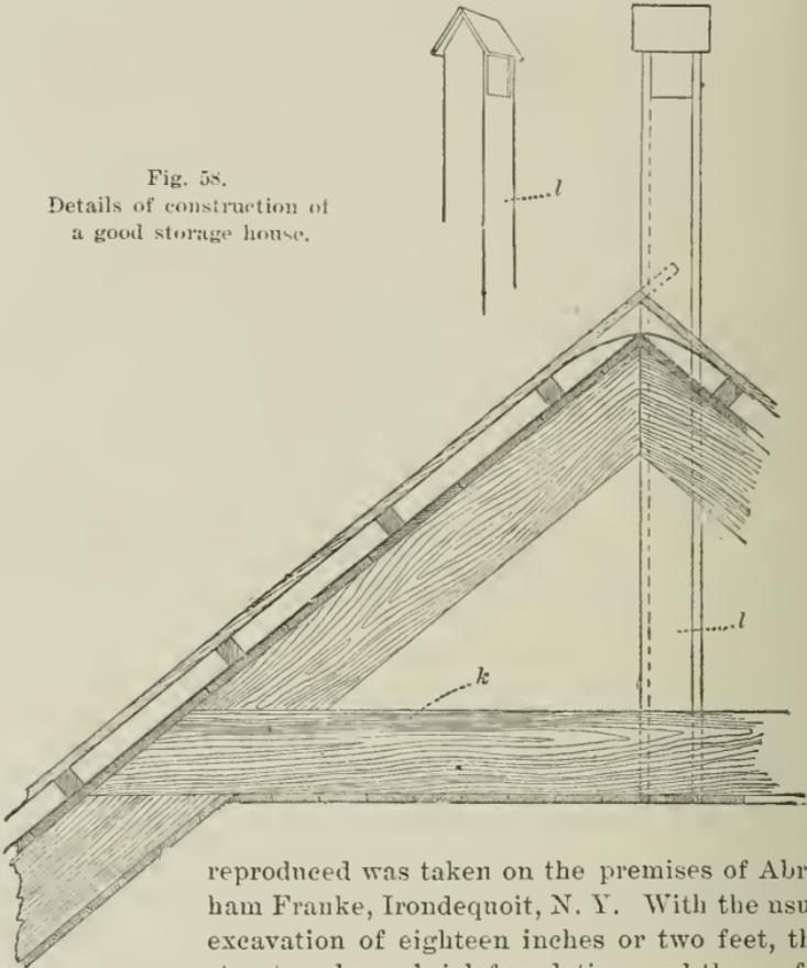
reproduced was taken on the premises of Abraham Franke, Irondequoit, N. Y. With the usual excavation of eighteen inches or two feet, this structure has a brick foundation, and the roof is well provided with air-chambers and paper linings, affording the best protection against cold. The additional large air-chamber above the collar-beams, with its separate windows, seems also desirable. There are large double doors at each end, and the
