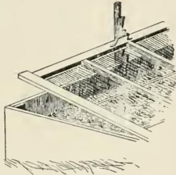
Fig. 23. Ventilating the hotbed.
