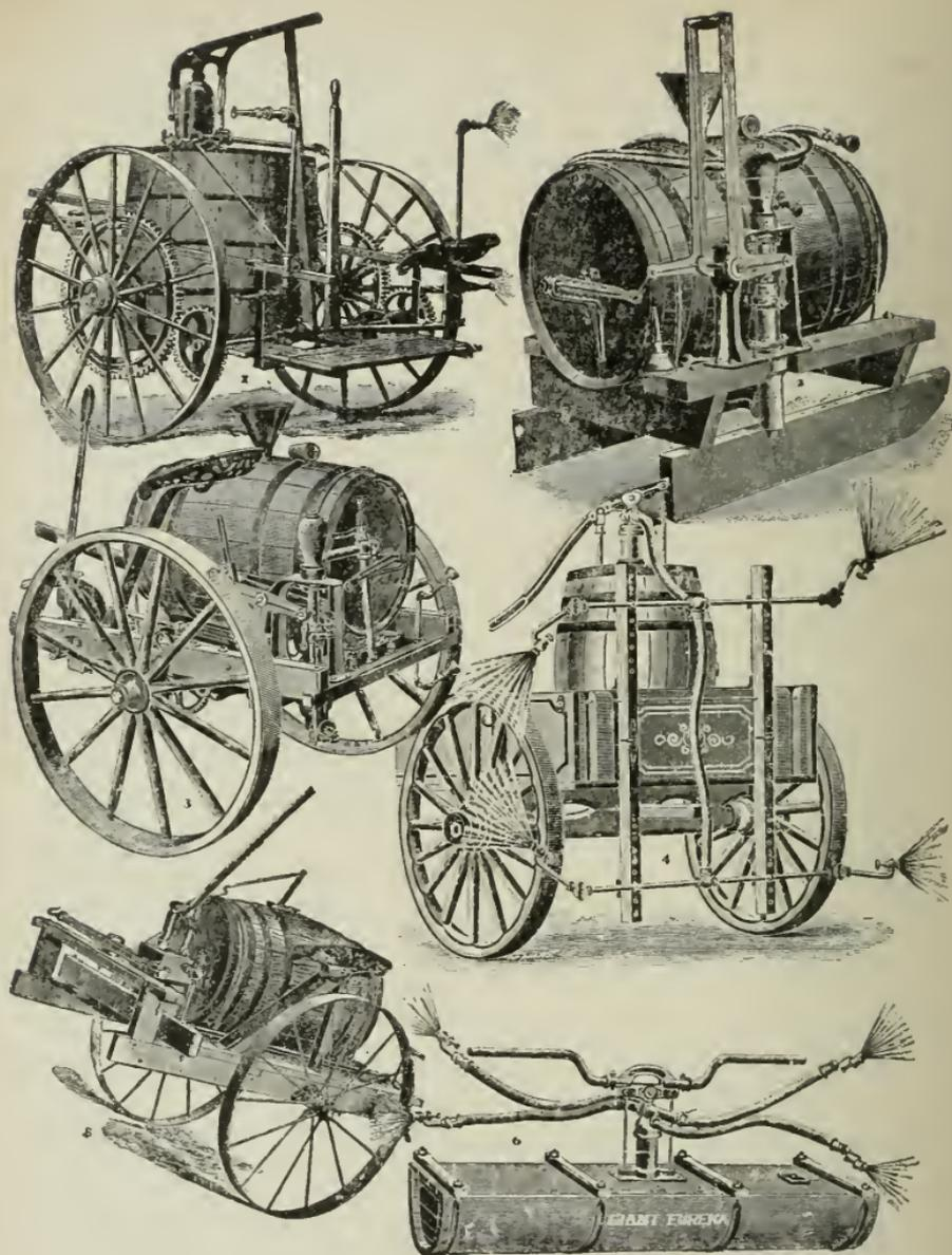
Fig. 48. Types of power and tank outfits.
