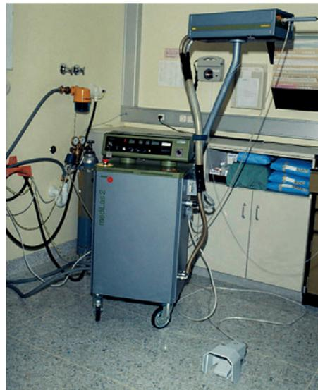
Fig. 19.1 Laser equipment, Nd:YAG laser (Medilas II, Dornier, Munich).
