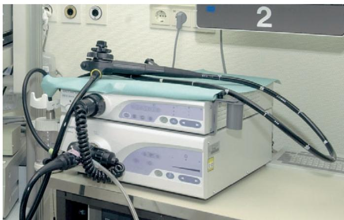
Fig. 2.9 Video processor (above) and light source (below) (courtesy of Mr. Wirth, photo archive, Augsburg Clinic).
