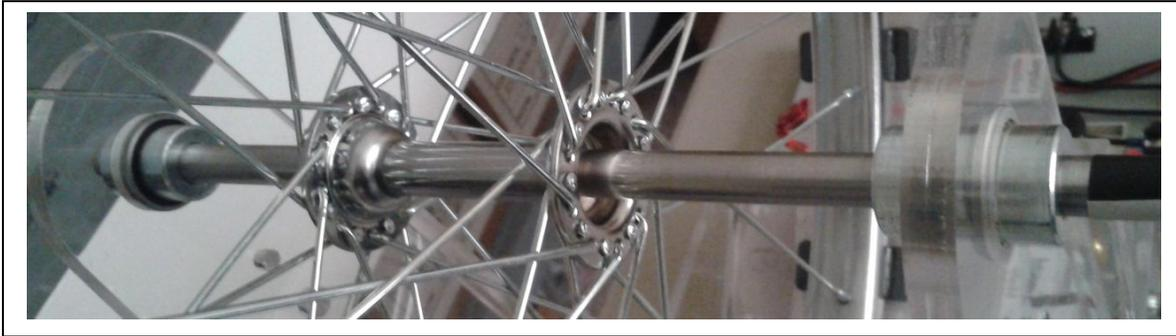
The next problem was the rim. With the hub running true, it was obvious how "out of round" the rim was. This required a laborious process of loosening and tightening the wheel spokes until all of the eccentricities were compensated. This took over an hour but was absolutely necessary.
