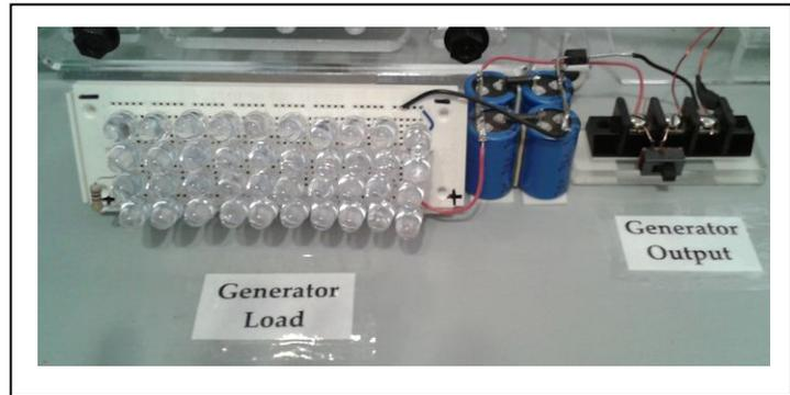
The switch was a simple toggle type. The diode was a 6A100. The four capacitors together had a capacitance of 470uf. The resistor was rated for 100 Ohms at one watt. The 40 LEDs were wired as 4 parallel strings of 10 LEDs connected in series.
