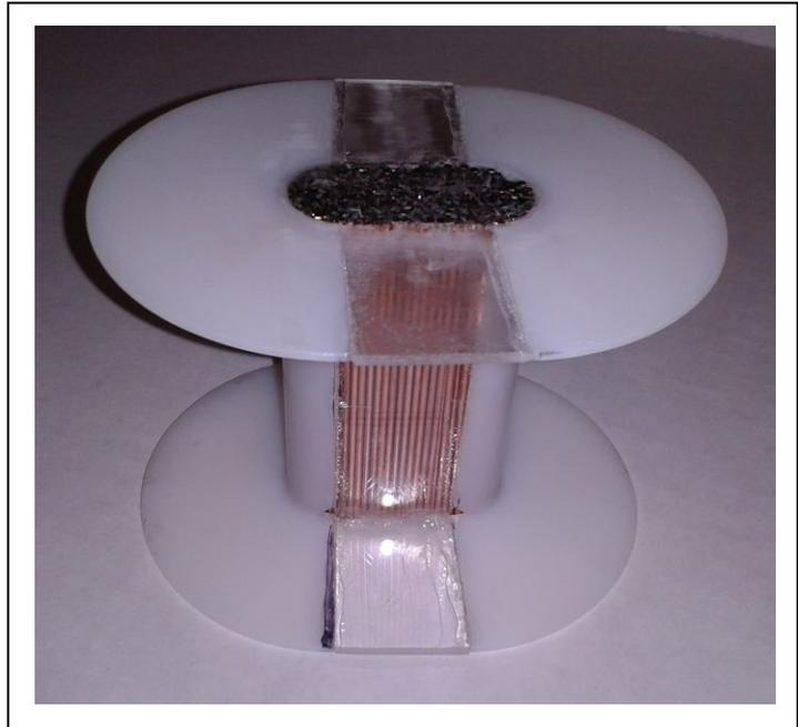
Once the coil form and core material were positioned, the iron rods were glued in place using cyanoacrylate (super glue) adhesive, similar to the process shown on page 61 of the **SG Beginner's Handbook**.
