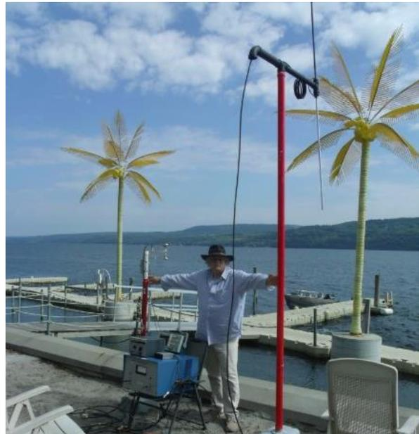
**Photo 3.** Propagation paths on Seneca Lake used by Burrows in 1936. In 2014 Corum used path 1. The photo shows the Zenneck probe (the small golden doublet, left side) mounted at six feet, and the conventional 52 MHz vertical  $\lambda/2$  dipole with a Guanella balun mounted at 10 feet (right side). Our 2014 data is shown in Figure 4, above. The Texzon technology described herein is Patent Pending.
