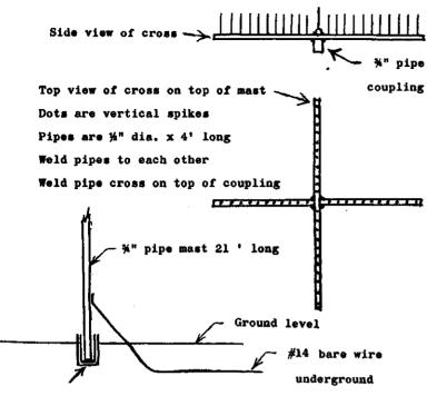
Glass jars 3 sizes Smallest one to fit %" pipe mast loosely That one inside of next one Second one inside of largest one
