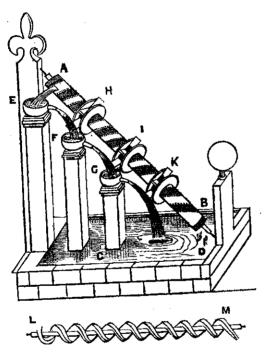
Where the figure L M, at the bottom, does represent a wooden cylinder with helical cavities cut in it, which at A B is sup-
