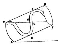
Where A B represents a screw covered over, C D E one helix or revolution of it, C D the ascending side, E D the descending side, the point D the middle; the horizontal line C F shewing how much of the helix is filled with water, viz., of the ascending side, from C the beginning of the helix, to D the middle of it; and on the descending side, from D the middle, to the point G, where the horizontal does cut the helix. Now, it is evident that this latter part, D G, is
