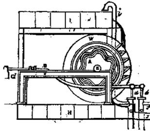
In connection herewith, a pump may be set in a tank of water, and a tank added above; on the same shaft with the face plate is a water-wheel driven by the water from above; when it
