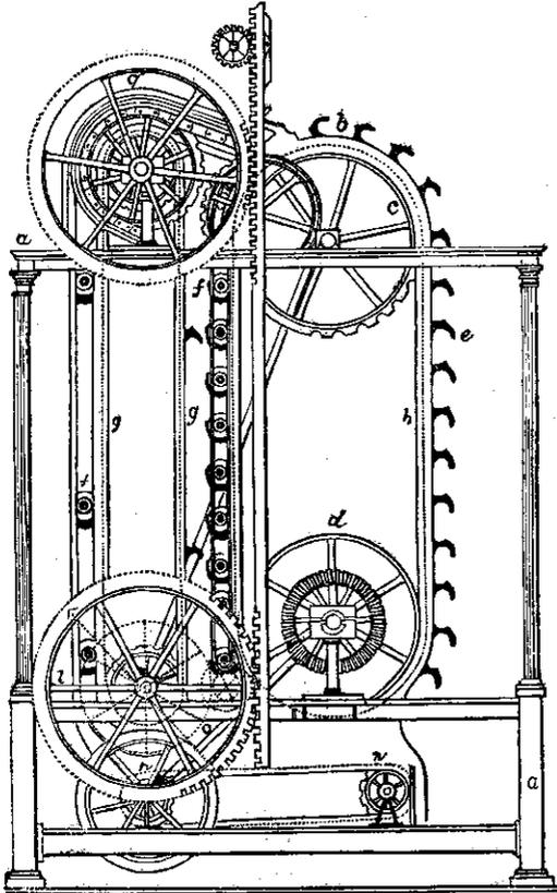
manner:—On the axis *c<sup>1</sup>* is affixed a bevelled toothed wheel *c<sup>3</sup>*, which takes into and drives the bevelled toothed wheel *k*
