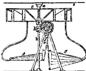
What I claim as my peculiar right is, the impulsion of a current of air against the fans of a drum (as that at *c*) through pipes, as at *d* and *e*) for the purposes of a motive power, together with a certain arrangement of mechanism, by means of which the action first induced shall be kept up.
