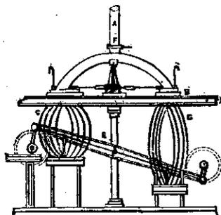
the main pipe, and which contains the column of water or other fluid, from the pressure or gravity whereof motive power is to be obtained. This pipe A is fixed to brickwork or in a general framework X, and terminates at the lower end in two branches  $A^1 A^2$ , whereof  $A^1$  leads into a chamber  $B^1$ , also fixed to the framework X, and perforated on
