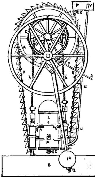
I do declare the nature of my said invention to consist in a machine, the nature of which depends on the descent of an endless series of reservoirs filled with water, which water is raised to a suitable elevation for the purpose, principally by the action of the machine itself.
