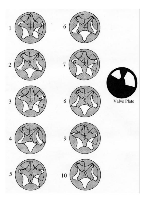
Figure 2. Porting for StarRotor compressor.
