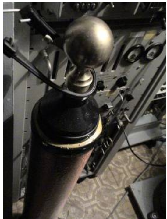
Tesla Coil: One of Hutchison's hand-wound coils for experimental testing.
