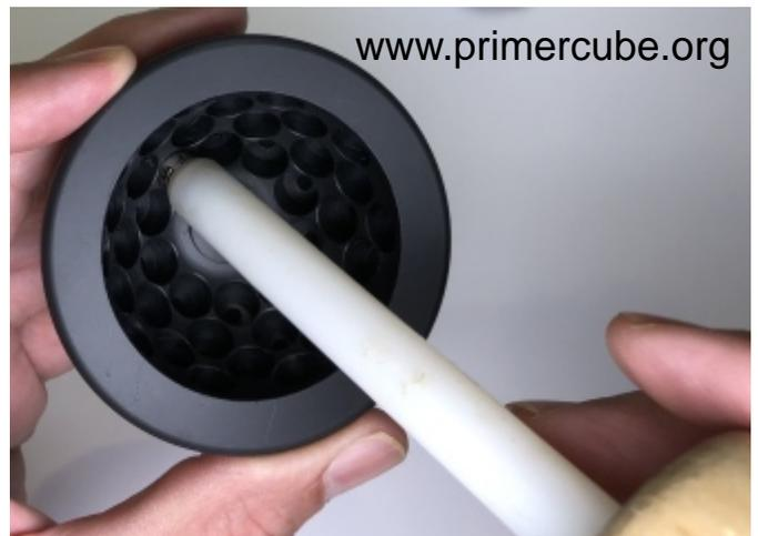
Insert the magnet into the hole until it bottoms out and then hold for a few seconds to allow the adhesive to cure.
