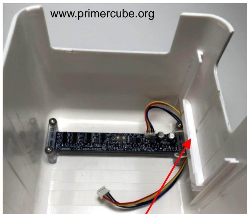
Attach PC 7080 to PC 7100 with Loctite 401 as shown above.
