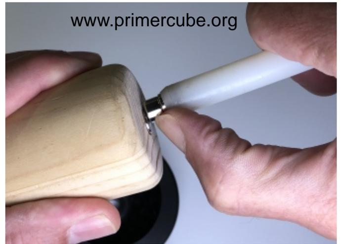
Use magnet insertion tool to remove one magnet from the stack.
