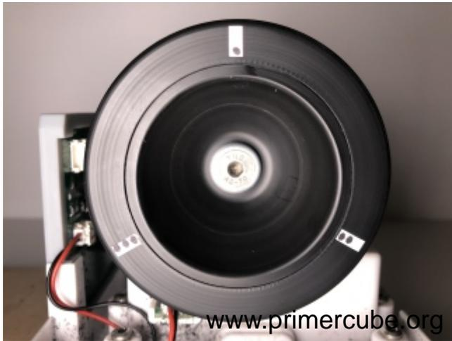
Above we see the rotor marked in three spots 120 degrees apart. The vibration level is measured while the rotor is running at 3350 RPM
