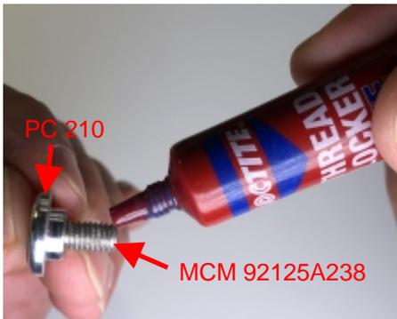
Insert screw # MCM 92125A238 into PC 210 and then put a drop of threadlocker on the screw.
