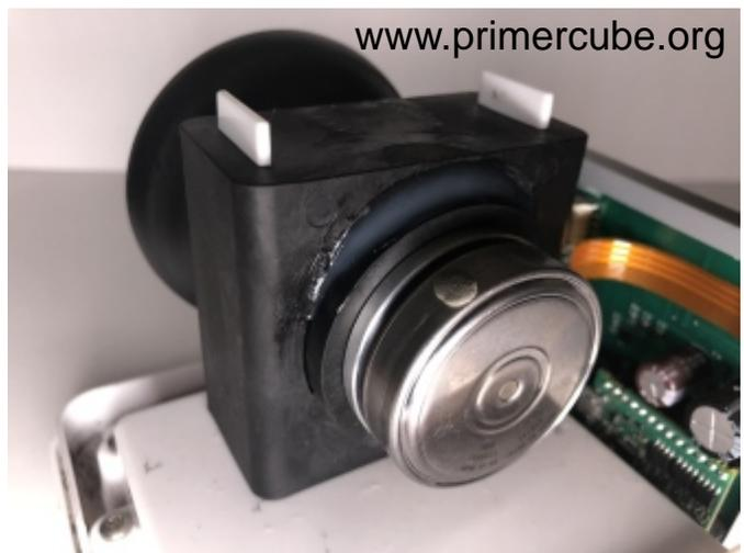
After a bit of fine tuning we have the proper weight and location of the two temporary clay balancing weights required for a smooth running rotor. The photo to the right shows the temporary balance weight on the motor, but some rotors do not need this balancing weight as they are smooth enough with just the balancing weight on one side of the bearings.
