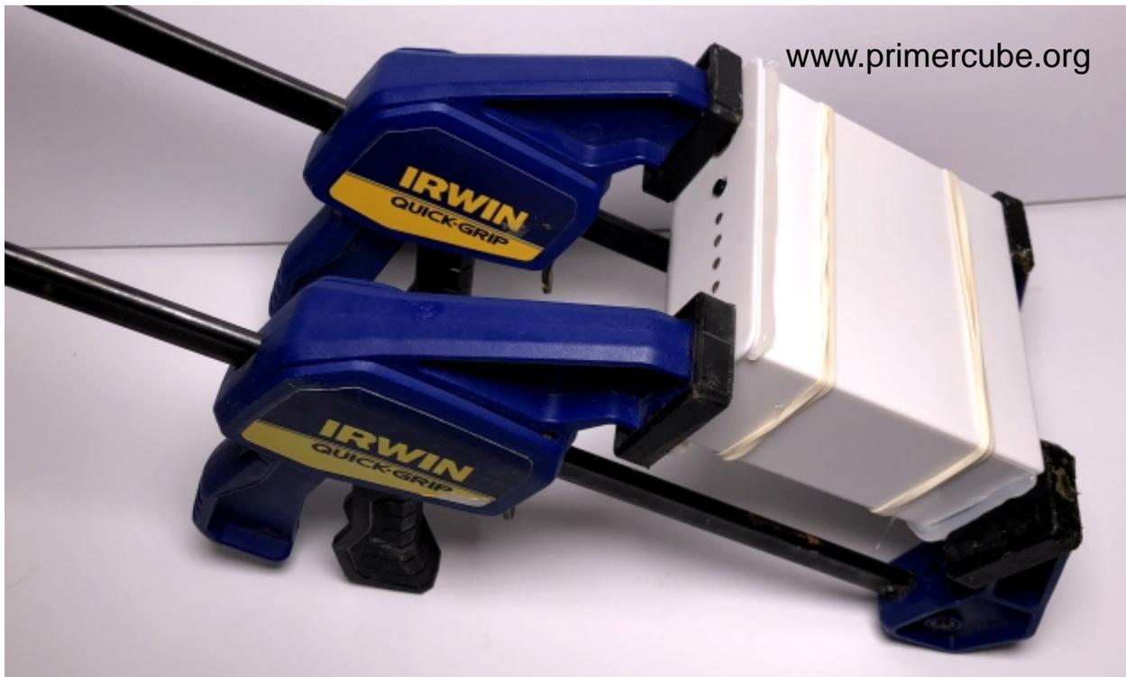
Apply clamps and squeeze out excess GE 5100 silicone. After allowing the silicone to cure for three hours the excess silicone can easily be removed. This completes the battery pack.
