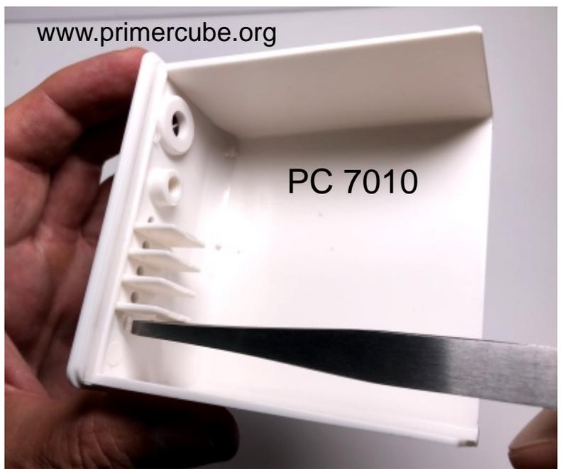
Hold PC 7040 with tweezers and apply Loctite 401 sparingly as shown above. Then carefully insert PC 7040 into place and hold for a few seconds for the adhesive to set. Repeat for the other four PC 7040. It should look like the image below when finished.
