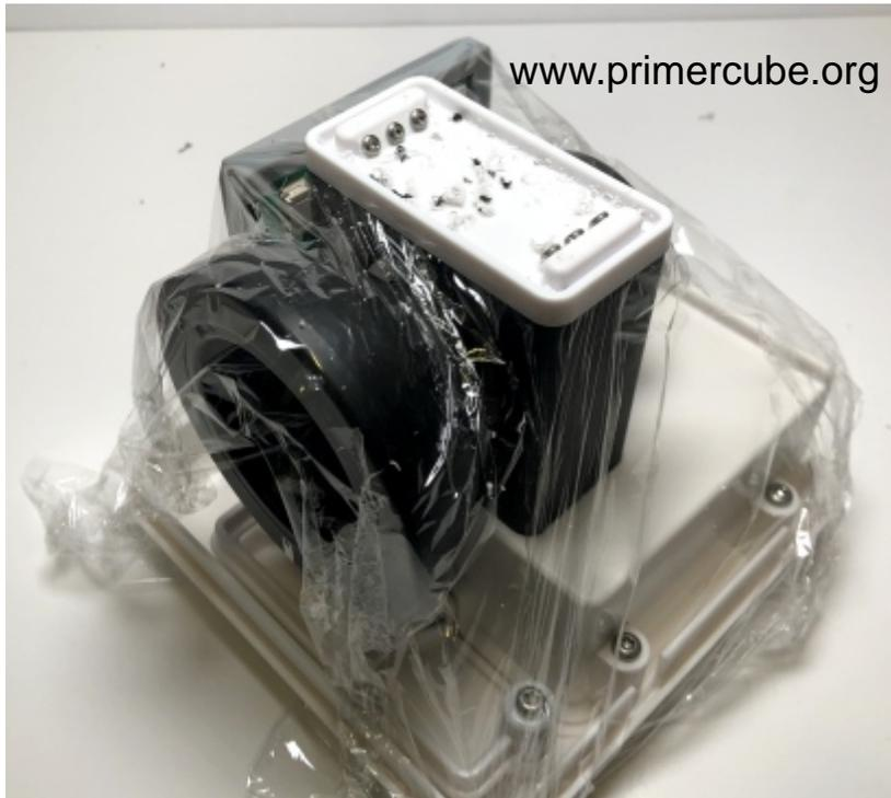
The above photo shows the six McM 96001A156 screws in place. Remove the shavings and then remove the plastic wrap.
