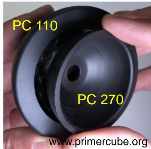
Make sure that PC 200 is fully seated then place part # PC 270 into PC 110. **\*\*ASSEMBLY TIP\*\*** Although not required it is desirable to put a layer of silicon sealant such as GE5100 on top of the magnets before PC 270 is inserted into PC 110 as this helps keep the magnets firmly in place. A loose magnet can lead to undesirable vibration.
