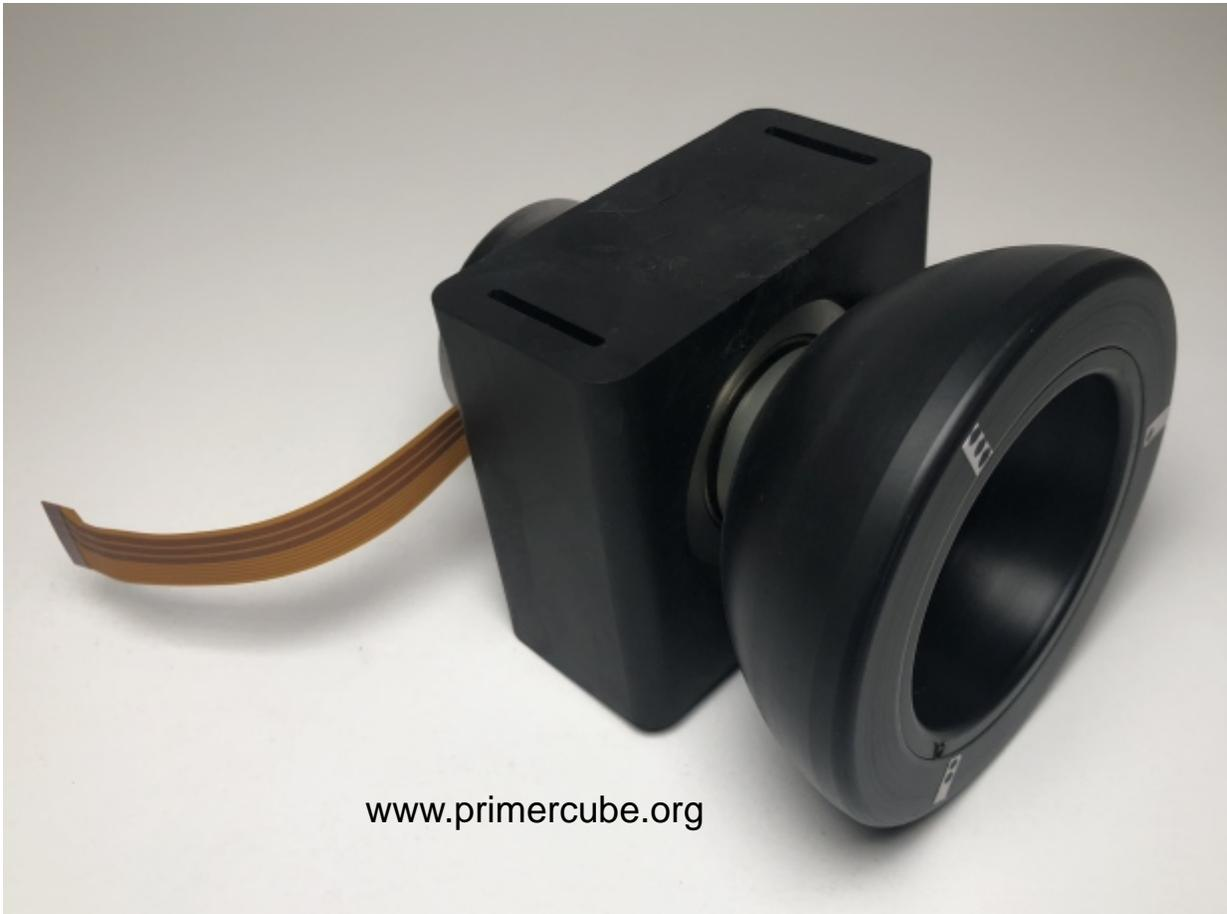
A completed PrimerCube rotor/motor assembly balanced, tested and ready to install on the mounts in a production PrimerCube.
