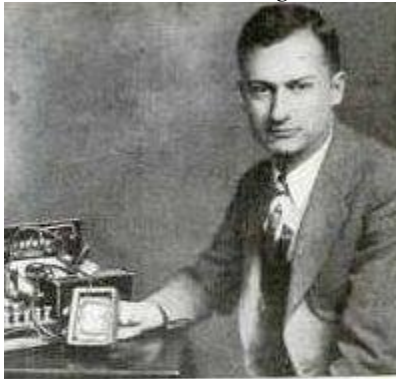
Batteries and vacuum tubes in radio sets may become a thing of the past, with this amazing invention of Dr. Palmer H. Craig, of Cincinnati. Bismuth plates, it is said, generate the energy to operate the radio set, and serve as detector and amplifier
