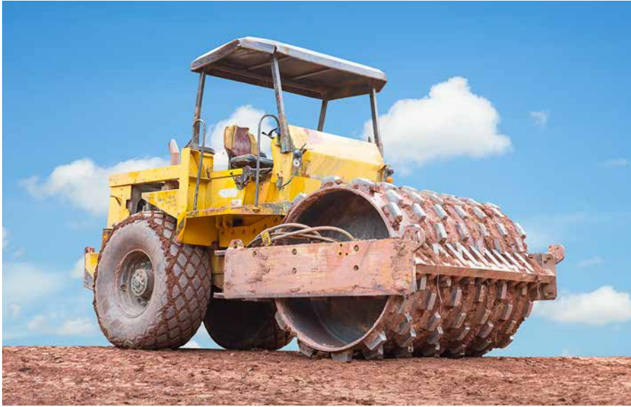
FIGURE 5.4. A padded-drum compactor.
