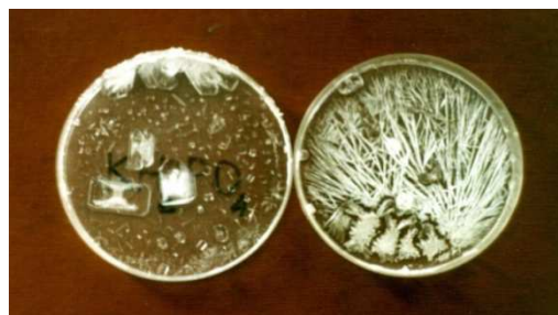
Fig. 3. KH_2PO_4 crystals. Left: the evaporation of solutions from the anode department of the electrolyzer formed crystals of the cubic form; right: the evaporation of solutions from the cathode department – the needle-shaped crystals.
