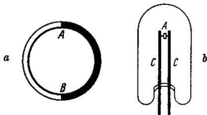
If the junctions are maintained at different temperatures, a current will flow in the circuit, which is proportional to the temperature difference of the two junctions. Modern high-sensitivity thermopiles are frequently built as diagrammed in fig. 16b in
