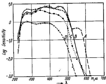
Figure 17. Spectral sensitivity curves of Eastman plates
