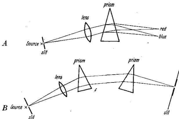
Figure 15. Spectrometers
