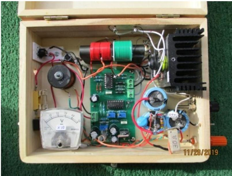
**Fig. 7.6.** Capacitor charger built on the circuit shown in Fig. 7.5
