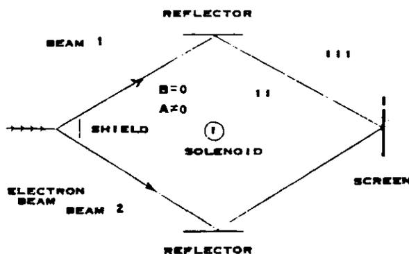
Fig. 1 Set-Up for Aharonov-Bohm Interference Experiment
