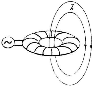
Fig. 2 Toroid  $\vec{A}$  Field Generator
