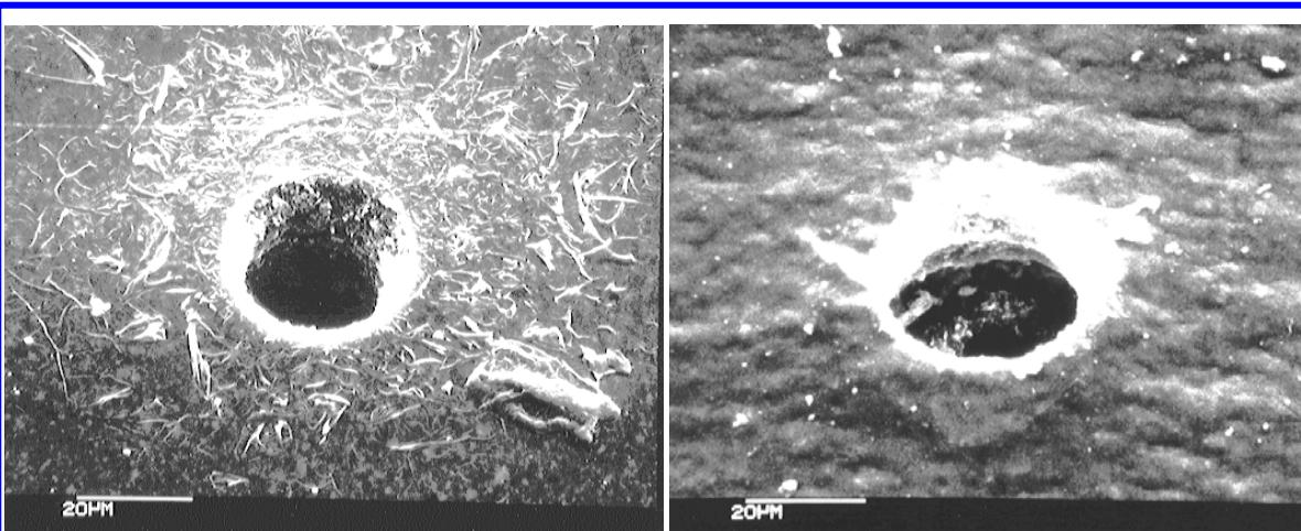
Fig. 12 Entry side of an EV strike on silicon carbide grain
