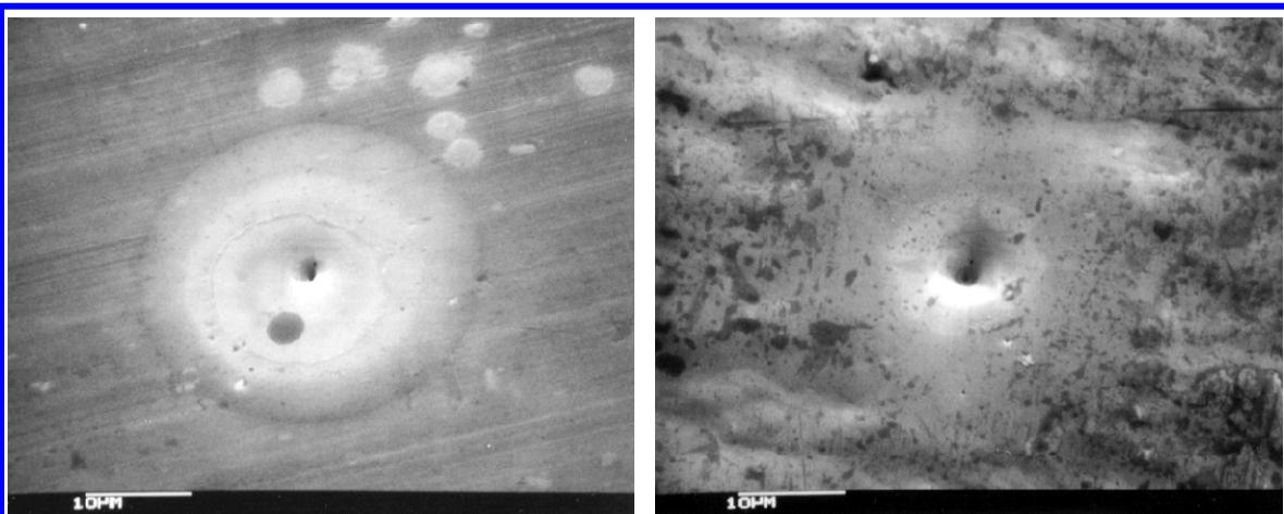
Fig. 1 EV strike on 6 micrometer thick aluminum foil.
