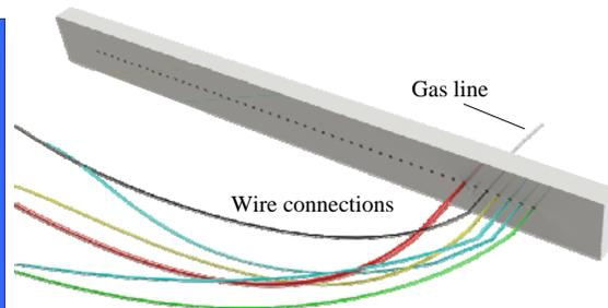
Fig. 9 Ceramic connector block with 7 of the 50 available wires or gas lines inserted.
