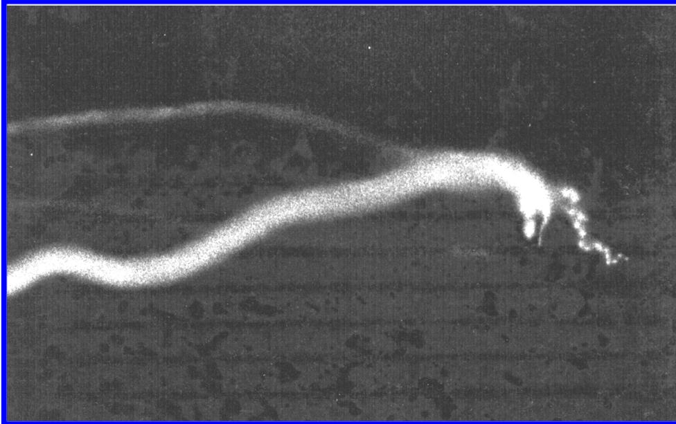
**Fig. 1 EVO Strike with Skipping on Anode in Xenon Flash Tube Powered by Piezoelectric Generator.**
