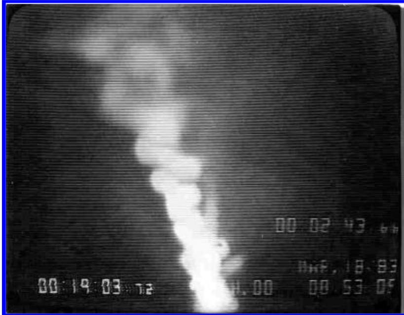
**Fig. 5 Pinhole Camera Side View of Dual EVO Flight Through Vacuum.**
