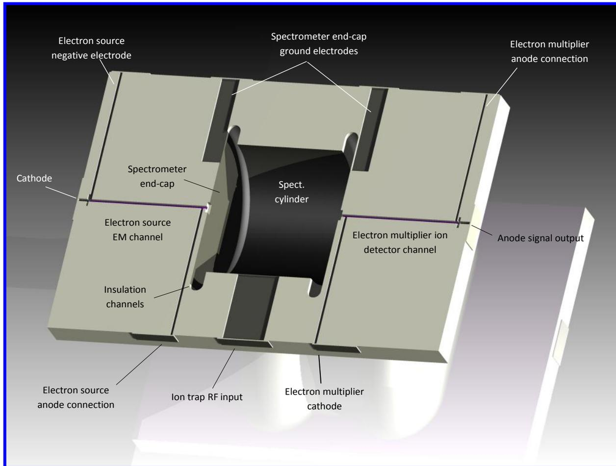
View of active side of cast ceramic ITMS showing electron multipliers and spectrometer cylinder. Two similar plates are assembled to form a complete spectrometer. Several of these small mass spectrometers can be used simultaneously in an experiment.
