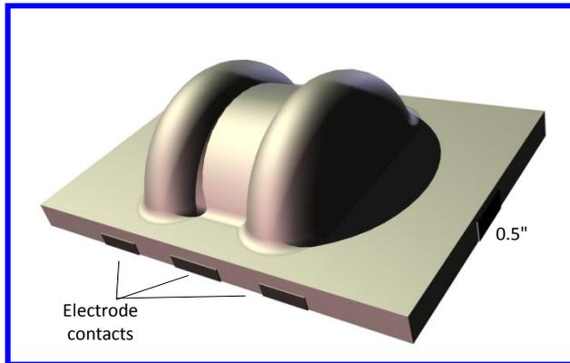
Top view of cast ceramic ITMS shell showing electrode contacts and basic dimension
