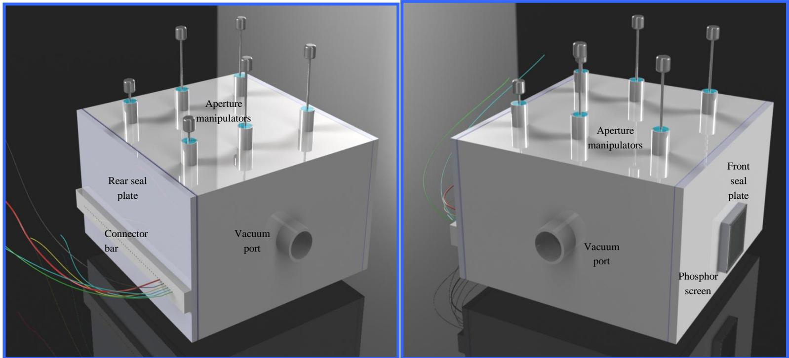
Two views of the outside of the basic experimental chamber which houses all of the major instruments for analysis of the results of both EVO action and its effect on nearby material. The container is made from cast alumina ceramic and then glazed. Of all the components in this proposal, this unit is the one that is modified more often than any other.
