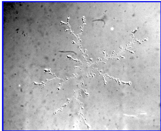
Photo 2: Optical photo of witness plate taken at 1,500X showing EVO swarm connected as bead chain structure.
