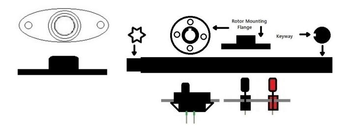
Bearings, 2 Mounting Flanges for the Rotor to be attached to a Shaft with one end machined to match the Pull Starter Socket.
