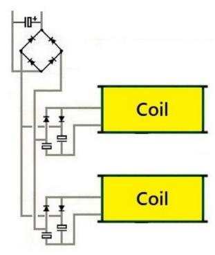
The Power Recovery Circuit allows energy to be collected from the rising and falling magnetic field of the remaining coils on the rotor.
