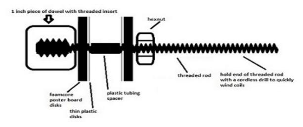
into the Insert. Slip one Foamcore Disk onto the Rod pushing down to the block of wood followed by one Thin Plastic Disk, one Spacer Tube, another Thin Plastic Disk, another Foamcore Disk and finish by screwing on the Hexnut all the way down to the Coil form. Screw it down
