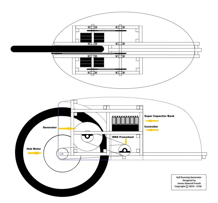
This next adaption of my Generator has multiple uses. The Counter Rotating Sections eliminate most of the torque created by the centrifugal force of a large spinning mass.
