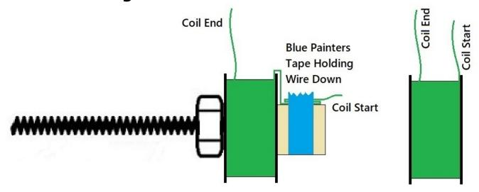
Hold the wire between the Winder and the Wire Spool with a folded up paper towel, your fingers will thank you for it. Start the drill slowly increase the speed as you get the hang of winding the coils.
