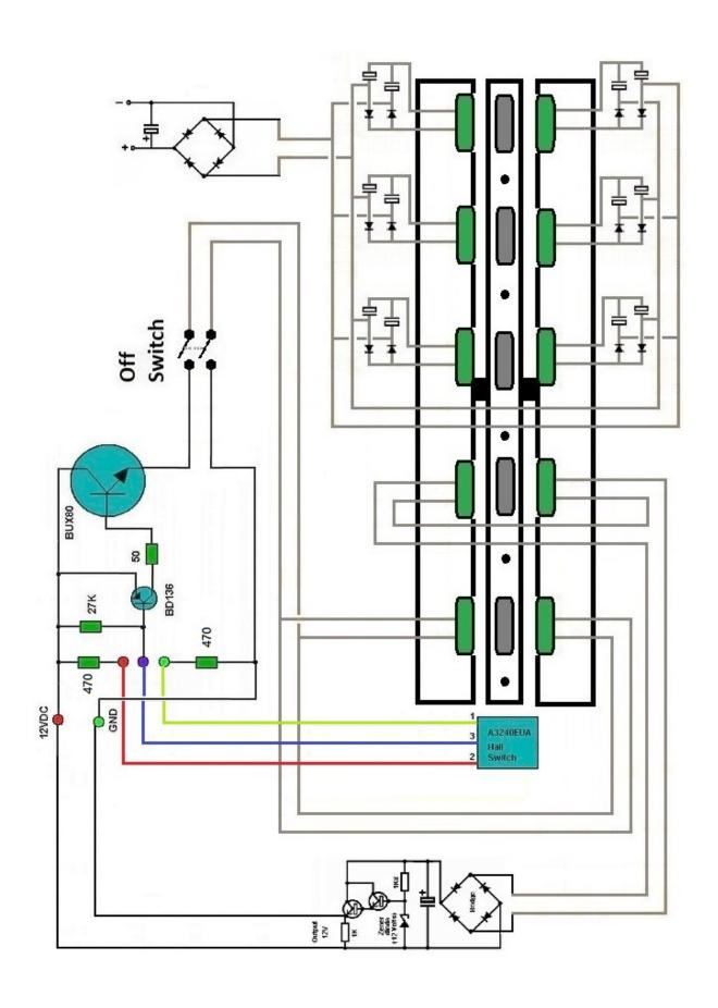
The power created needs to be fed into an Adjustable Regulated Power Supply and be adjusted to put out 12 volts DC. This must be done while the generator is running. This adjustment only needs to be done once when the assembly of the Generator is finished. Hooking up a Power Inverter to the output terminals will produce 120 volts AC.
