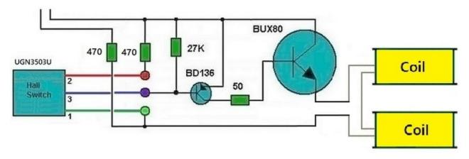
The Hall Switch is best described as a magnetic lock. A magnetic field coming close to it is the key that opens the lock allowing current to flow. Embed small round bar magnets in the rim of the rotor and mount the hall sensor close to the rotor's rim.
