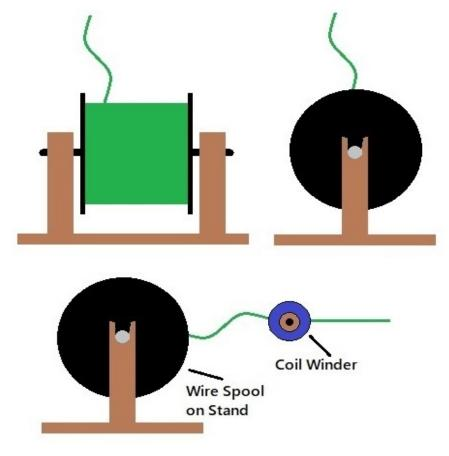
Take the Coil winder put in a cordless drill like you would with a regular drill bit. Pull about 2 feet of wire off the
