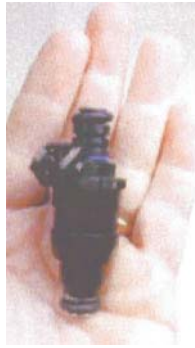
Fig.2 The Accel high impedance fuel injector used in our experiment.
