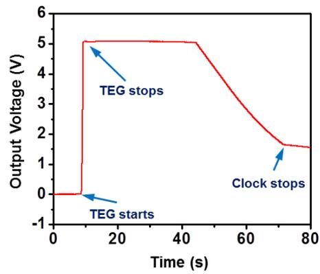
**Supplementary Figure 6 | Output voltage of the power-supplying system when powering a digital clock.** For the triboelectric generator rotating for less than 1 sec at  $3000 \text{ rmin}^{-1}$ , the system can sustain continuous operation of the clock for 60 seconds.
