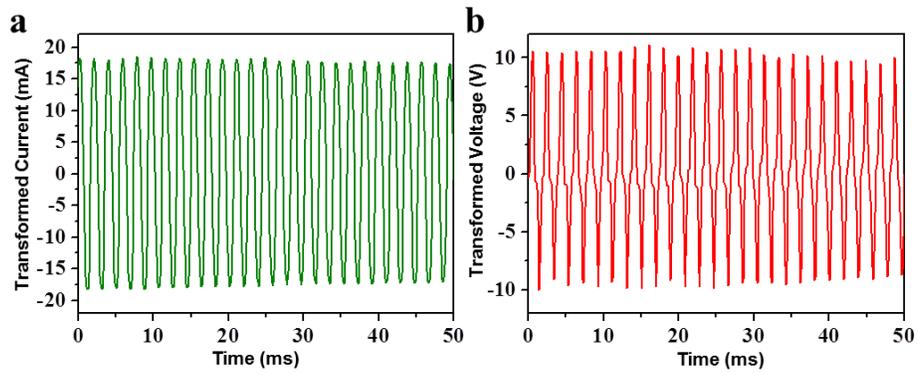
**Supplementary Figure 4 | Transformation of the electric output by a transformer. (a)** Enhanced output current without external load at a rotation rate of  $500 \text{ rmin}^{-1}$ . **(b)** Reduced output voltage without external load at a rotation rate of  $500 \text{ rmin}^{-1}$ .
