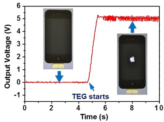
**Supplementary Figure 7 | Output voltage of the power-supplying system when charging a cellphone.** For the triboelectric generator rotating at  $3000 \text{ rmin}^{-1}$ , the cellphone turns on automatically as soon as the output voltage reaches 5 V.
