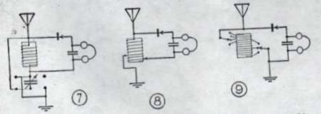
comb coil. With the condenser in series, no wavelength can be obtained as great as if the condenser were omitted, and the lower the capacity used, the shorter will be the wave to which the set is tuned.
