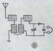
antenna coil by either a slider or switches, but since the closed circuit winding is arranged to be rotated, merhanical difficulties make variations in the inductance of the secondary practically out of the question. For that reason all of the tuning in the secondary circuit is accomplished by means of the variable condenser shunted across the winding.
