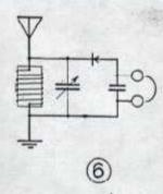
is desired. The telephone and detector are placed in series across the inductance for the purpose of rectifying and converting into sound the wave trains traveling thru it. This is a marked improvement over circuit No. 1, for the high resistance detector is removed from the antenna circuit, and the tuning coil permits adjustments to various wavelengths without undue interference from others. This circuit is employed in most of the lower priced receiving outfits now marketed for
