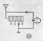
24. A type of antenna not previously referred to is illustrated in this circuit. It is termed a loop antenna but must not be confused with the coil type or directional loops, for it is as efficient as the ordinary aerial and is no more directional. Such an antenna with its attendant tuning arrangement was championed by De Forest in the early days of wireless development and tound considerable favor among experimenters at that time.
