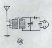
18. This circuit depicts the usual crystal detector, telephones and stopping condenser, connected to a loosely coupled two circuit tuner whose secondary inductance is of fixed value while the primary is varied by means of units and tens awitches. A tener of this type is usually built so that the coupling between the cools is varied by rotating the secondary inside the primary tube, and is commonly referred to as a vario coupler. It is a simple matter to vary the inductance of the
