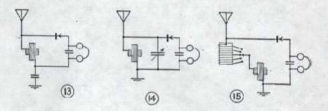
from its position of minimum inductance toward the opposite end until the desired wavelength is obtained. It is well to mount the two coils at right angles and several inches spart so that when the loading coil is not required, losses which would other wise be high on wavelengths near its natural period will not be so greatly felt.
