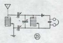
20. The circuit here shown is that of an extremely selective loosely coupled receiving tuner having three circuits. The antenna circuit includes a variable condenser and an inductance which is inductively coupled to a coil of an intermediate circuit. The intermediate circuit is tuned to resonance with the antenna circuit by means of a variable capacity, and has a second inductance which is variably coupled to the detector circuit. In this case the detector circuit is aperiodic.
